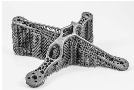
Figure 1.19: Difficulty in the removal of support structure without damage[STA 17]
