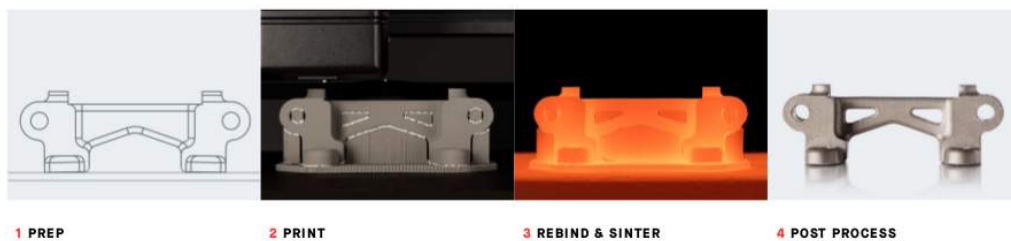
Figure 1.1: Bound Metal Deposition[MET 17]
