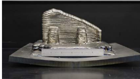
Figure 1.18: Wrapping of substrate after AM fabrication[ZEL 15]
