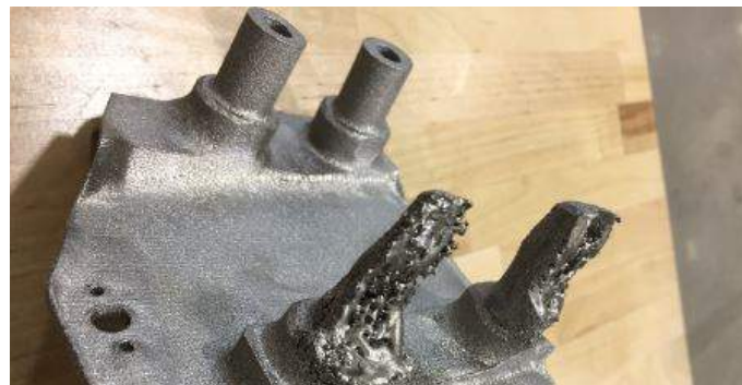
Figure 1.16: Incompleted parts induced by lack of fusion[MCG 17]
