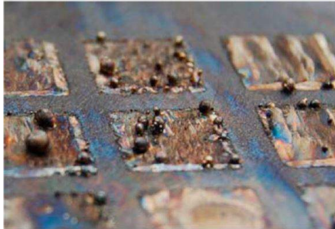
Figure 1.17: Balling effect on part's surface in EBM, caused by overheating[ZÄH 10]
