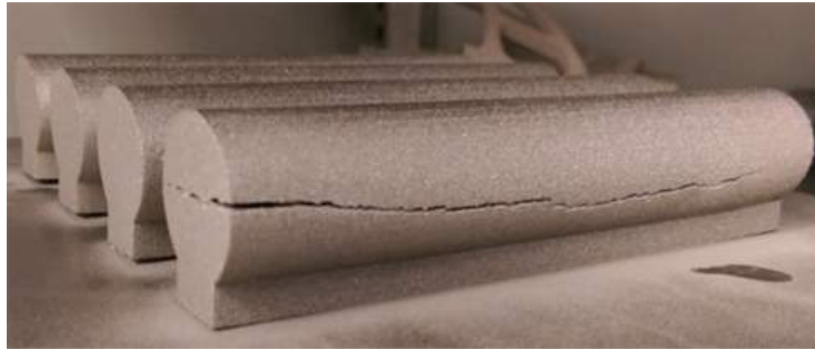
Figure 1.10: Crack caused by residual stress[COM 17]
