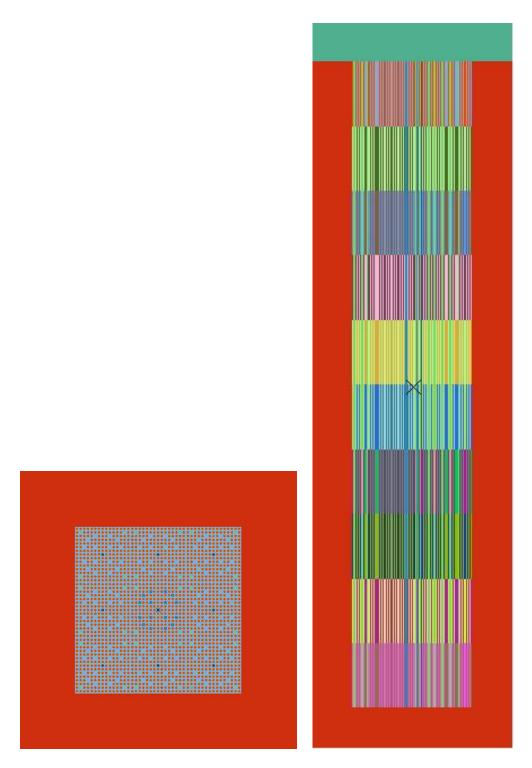
Figure 3.7 – Views of the ROOT implementation of the TMI-1 mini-core geometry. Each color defines one composition. Left: radial cut with the central assembly with control rods (in blue). The burnable poison pins are represented in green. Right: axial cut.
