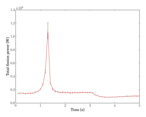
Figure 6.15 – Time evolution of the total power (in watts) in the TMI-1 3x3 mini-core computed with T4/SCF during scenario C transient, where control rods are progressively extracted by 40 cm between t = 0.3 s and t = 1.3 s and reinserted back to their initial position between t = 3.1 s and t = 4.1 s.
