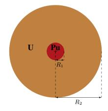
Figure A.1 – A 2-D cross-section view of Flattop-Pu, a plutonium sphere with a natural uranium reflector.
