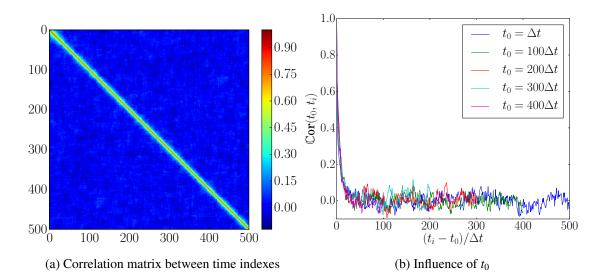
Figure 3.13 – Two-time correlation function for the rod drop subcritical configuration ( $\rho \approx -19$  \$). The total neutron flux was collected over 500 time steps with TRIPOLI-4.
