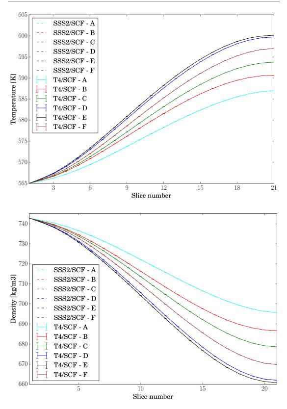
Figure 5.4 – Coolant temperatures and densities obtained with T4/SCF (solid lines) and SSS2/SCF calculations (dashed lines), for the six channels of the TMI-1 assembly identified in Fig. 5.3, at the inlet of each slice. Slice number 1 is located at the bottom of the assembly. Top: coolant temperature profiles in 6 channels. Bottom: coolant density profiles in 6 channels.
