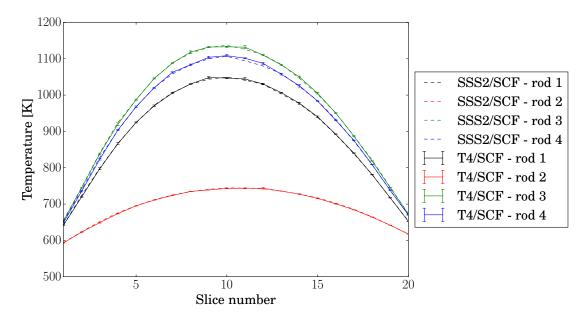
Figure 5.7 – Axial fuel temperature profiles obtained with T4/SCF (solid lines) and SSS2/SCF (dashed lines).
