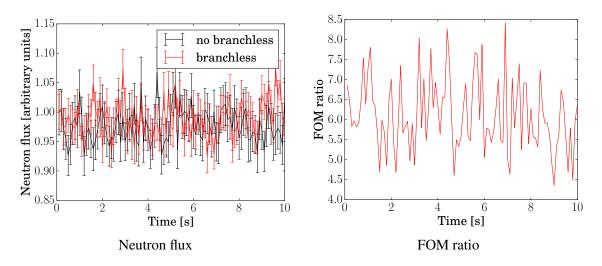
Figure 2.10 – Time evolution of the total neutron flux in TMI assembly with and without branchless method. The source is prepared in a critical state. Left: Total neutron flux. Right: FOM ratio between simulations with/without branchless collisions.
