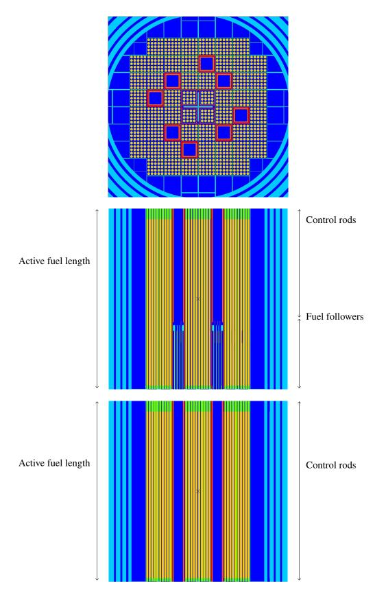
Figure 3.1 – Top: radial cut of the TRIPOLI-4 model for the operational loading of the SPERT III E-core at mid-plane. Middle: axial cut of the TRIPOLI-4 model, passing through two control rods. The lower portion of the control rod is a fuel follower, and the upper portion (orange) is the absorbing section. In between lies a flux suppressor. Bottom: axial cut of the TRIPOLI-4 model, passing through two fully inserted control rods, corresponding to the shutdown configuration.
