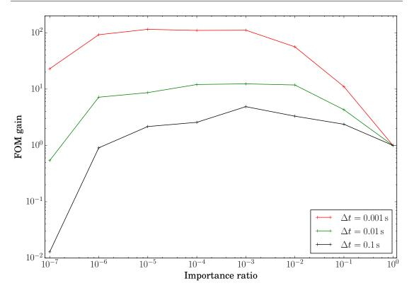
Figure 2.15 – Gains of figures of merit with respect to the calculations without importance sampling, as a function of the importance ratios.
