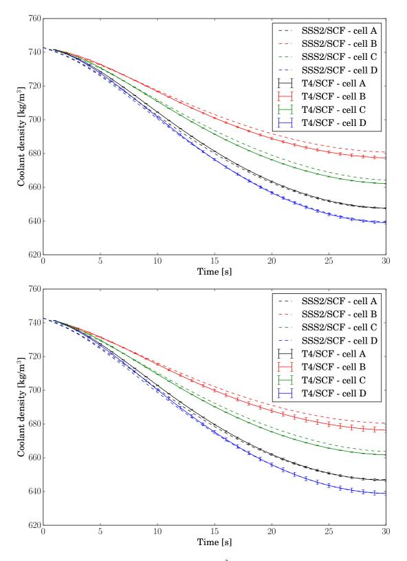
Figure 6.13 – Axial coolant density profiles (in kg/m<sup>3</sup>) for cells A to D in the TMI-1 3x3 minicore computed with T4/SCF (solid line) and SSS2/SCF (dashed line) between t = 1.1 s and t = 1.2 s. Note that the coolant temperature and density values for SSS2/SCF values are taken from one of the neighbouring channels. Top: 30 cm rod extraction. Bottom: 40 cm rod extraction.
