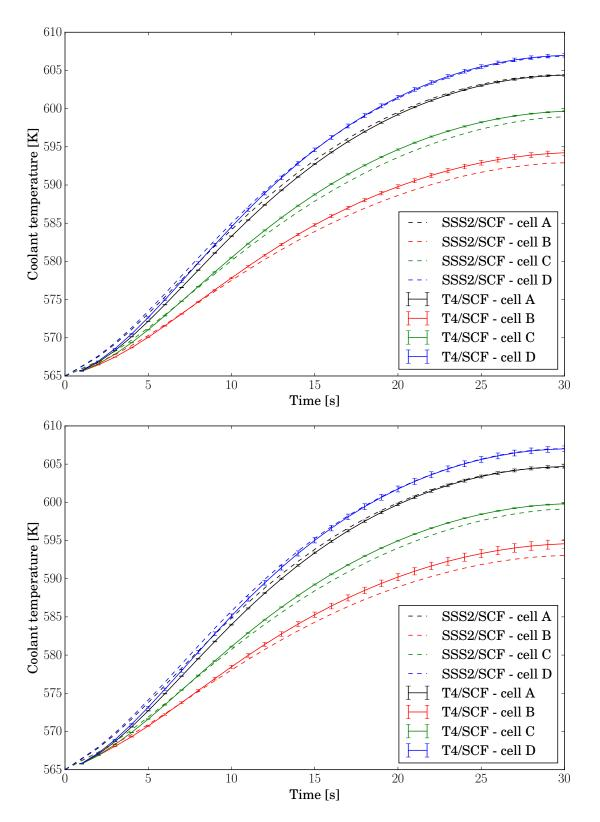
Figure 6.12 – Axial coolant temperature profiles (in kelvins) for cells A to D in the TMI-1 3x3 mini-core computed with T4/SCF (solid line) and SSS2/SCF (dashed line) between t = 1.1 s and t = 1.2 s. Note that the coolant temperature and density values for SSS2/SCF values are taken from one of the neighbouring channels. Top: 30 cm rod extraction. Bottom: 40 cm rod extraction.
