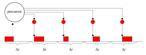
Figure 2.4 – Scheme of the forced decay with one precursor. The precursor is forced to decay in each time bin  $\Delta t$ , so that each time bin is filled with neutrons.
