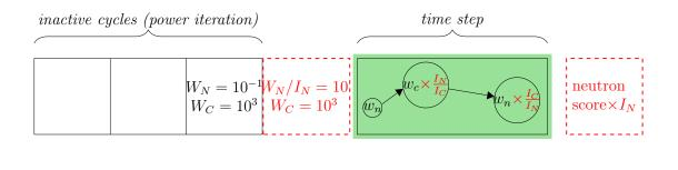
$\square$  criticality source computationapplication of the importance ratio  $R = 10^{-2}$ kinetic simulation $(I_N \approx 10^{-2}, I_C \approx 1)$
