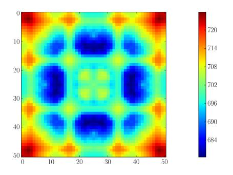
Figure 6.2 – Coolant density map (in kg/m<sup>3</sup>) obtained with T4/SCF for the TMI-1 3x3 minicore, averaged across all axial slices. The densities are used as initial values for the dynamic calculations.
