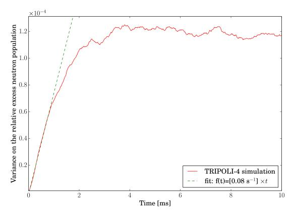
Figure 8.2 – Time evolution of the variance on the neutron population, for the TRIPOLI-4 simulation presented in Sec. 3.3.1. The plot is divided in two parts: the variance of  $N_t$  depends linearly on time up to  $t \approx 1$  ms, then it reaches a plateau.
