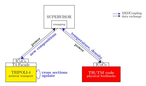
Figure 4.1 – Architecture of the supervisor-driven calculations performed using T4\_Facade class, the ICoCo API and the MEDCoupling library.
