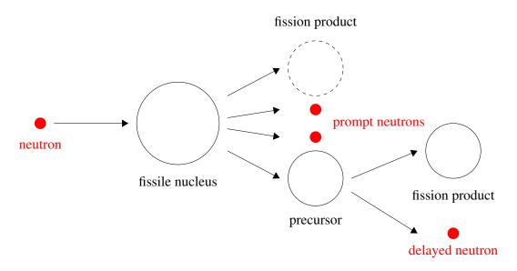
Figure 1.2 – Schematic depicture of neutron-induced fission with the different particles produced. After the fission, prompt neutrons and precursors are emitted almost instantaneously while delayed neutrons are emitted after precursors decay.
