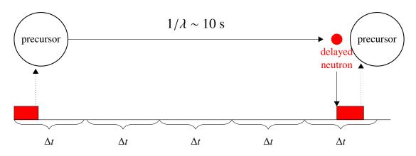
Figure 2.3 – Scheme of the analog process of precursor decay with one precursor. When the precursor finally decays, only one time bin is filled with a delayed neutron: this leads to variance jumps in the different time bins.
