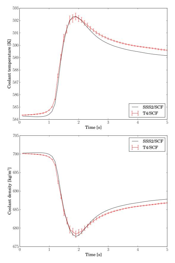
Figure 6.10 – Time evolution of the coolant fields in the TMI-1 3x3 mini-core computed with T4/SCF (red line) and SSS2/SCF (black line) with the control rods progressively extracted by 40 cm between t = 0.3 s and t = 1.3 s. Top: average coolant temperature (in kelvins). Bottom: average coolant density (in kg/m<sup>3</sup>).
