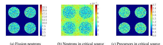
Figure 2.1 – Histogram of the particle weights in a 2x2 array of pin cells. Left: fission neutrons
