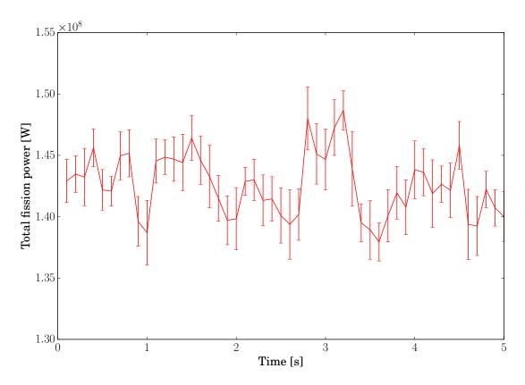
Figure 6.5 – Time evolution of the total power (in watts) in the TMI-1 3x3 mini-core computed with T4/SCF in steady-state conditions. The total power is stable and fluctuates around 140.94 MW.
