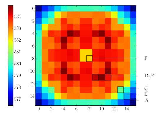
Figure 5.3 – Coolant temperature map (in kelvins) obtained with T4/SCF for the TMI-1 assembly, averaged across all axial slices.
