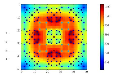
Figure 6.3 – Fuel temperature map (in kelvins) obtained with T4/SCF for the TMI-1 3x3 minicore, averaged across all axial slices. The temperatures are used as initial values for the dynamic calculations. Four rods are identified on the map for later analysis of simulation results.
