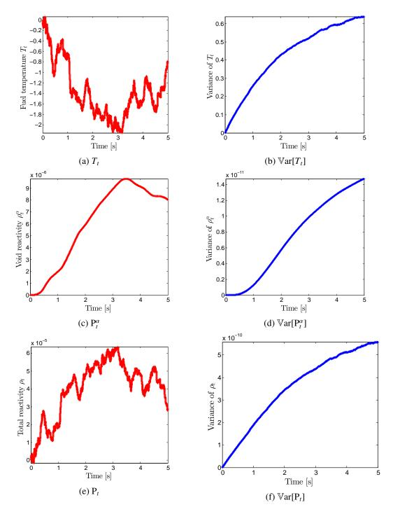
Figure 8.4 – Time evolution of the fuel temperature  $T_t$ , the void reactivity  $P_t^{\alpha}$  and the total reactivity  $P_t$  (red lines). Sample estimates of the variance of the three physical quantities are also plotted (blue lines). Results come from the same simulations as in Fig. 8.3.
