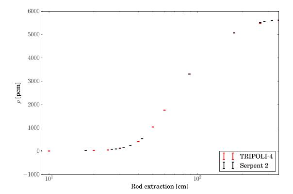
Figure 3.8 – Static reactivity as a function of control rod extraction for the TMI-1 mini-core. Criticality calculations were performed for several configurations: starting from critical configuration with complete insertion of the control rods in the core, up to complete extraction. Red: TRIPOLI-4 simulation results. Black: Serpent 2 simulation results. Error bars are plotted but they are not visible because of the graph scale (standard errors are below 10 pcm).
