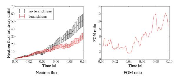
Figure 2.11 – Time evolution of the total neutron flux in TMI assembly with and without branchless method. The source is prepared in a critical state. At the beginning of the kinetic simulation, a reactivity of 1 \$ is introduced. Left: Total neutron flux. Right: FOM ratio between simulations with/without branchless collisions.
