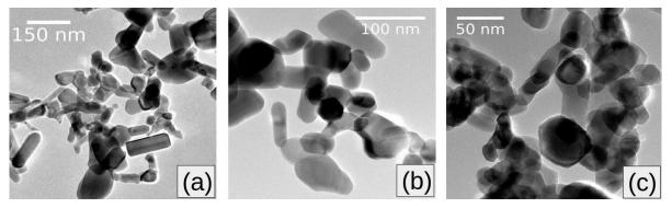
Fig. 3.1 Typical TEM images of (a) ZnO1, (b) ZnO2, (c) ZnO3 in ethanol [77].
