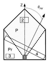
Fig. 5.1 The schematic representation of KDP crystals with pyramidal (P) and prismatic (Pr) sectors of growth,  $\theta_{PM}$  is the angle of synchronizm. 1 - initial crystal, 2,3 - samples of Z-cut of P and Pr of growth sectors, 4 - typical cut with maximum aperture.
