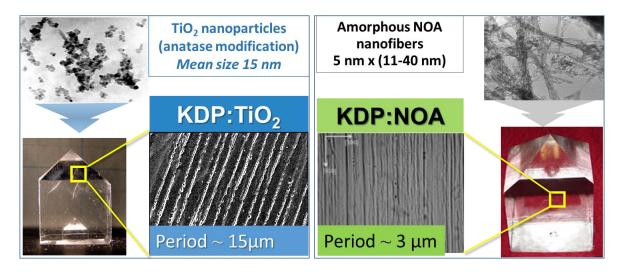
Fig. 5.2 Layered structure in composites based on the KDP matrix with incorporated  $TiO_2$  NPs and NOA nanofibers [48].
