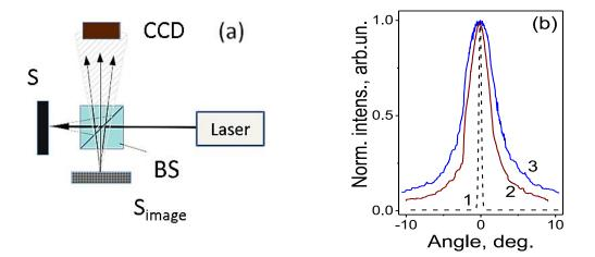
Fig. 2.2 (a) Scheme of extension to measure exact backscattering: *S*,  $S_{\text{image}}$  – sample and its image; BS – beam splitter; CCD – camera, photodiode or photomultiplier. (b) Manifestation of the self-defocusing effect in ZnO-II in the forward direction at a laser excitation intensity of 0.37 W/cm<sup>2</sup> (2) and 0.78 W/cm<sup>2</sup> (3), curve (1) corresponds to the free propagation of the laser beam [67].
