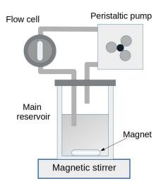
3.2.2 Measurement with colloidal suspension circulation system
