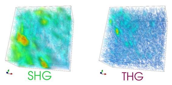
Fig. 2.8 3D reconstruction of SHG and THG signals from KTP microcrystals (~1 $\mu$ m) deposited on the glass substrate. Scanning range 10×10×6  $\mu$ m<sup>2</sup>.
