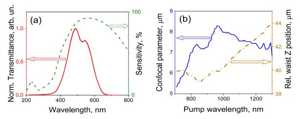
Fig. 3.14 (a) CCD camera spectral sensitivity (dashed curve) and optical system transmittance compensation curve (solid). (b) Confocal parameter (FWHM) (solid line) and waist position variation (dashed line) *vs* pumping wavelength.
