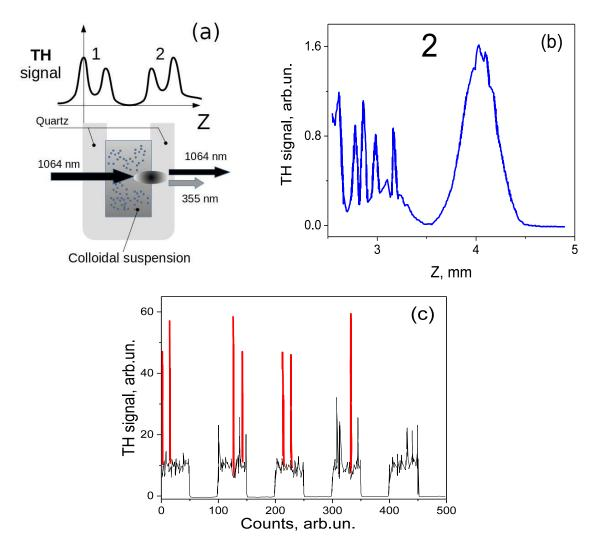
Fig. 3.2 Scanning of a static cuvette with a colloidal suspension of nanoparticles. (a) Schematic representation of the cuvette and response at the interfaces of colloid/quartz and quartz/air of the walls of the cuvette 1 and 2. (b) Scanned with a long averaging time (> 2 s) of the wall 2. (c) THG signal (pump beam modulated by chopper) with spikes that corresponds to the variable number of NPs in the waist and large agglomerates.
