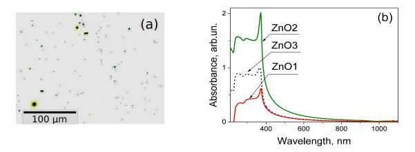
Fig. 3.9 (a) Optical image of internal surface of the flow cell after prolonged pumping of colloidal suspension. (b) Absorption spectra for ZnO nanoparticles with different sizes in ethanol.
