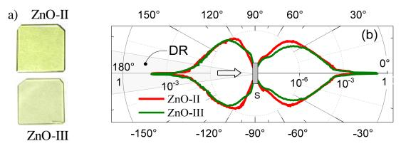
Fig. 2.3 (a) Photo of ZnO-II and ZnO-III crystals with different concentration of defects (b) Spatial distribution of elastic light scattering in ZnO crystals at 532 nm in polar coordinates (logarithmic scale on the radial axis). DR – exact backscattering region. S is the sample position. Arrow corresponds to the incident laser beam [67].
