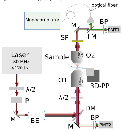
Fig. 2.7 Schematic representation of the experimental setup for multiphoton microscopy. P – polarizer;  $\lambda/2$  – half-wave plate; M – mirrors; BE – beam extender; BP – bandpass filters; DM – dichroic mirror; PMT1,2 – photomultipliers; O1,2 – objectives; 3D-PP – 3-axis piezoplatform (working range of 100 µm for three axes, minimum step 0.4 nm); SP – shortpass filter; FM – flipping mirror [95].
