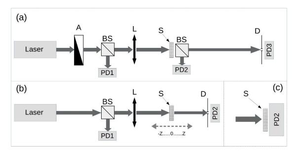
Fig. 2.6 (a) Optical scheme of the experiment for self-action analysis. A – optical attenuator; L - lens; BS – beam splitter; S – sample; D – diaphragm. Photodiodes: PD1 – reference, PD2 – total transmittance, PD3 – on-axis transmittance [87]. (b) is an example of an experimental scheme for Z-scan. (c) - modification of the setup (a) for accurate measurement of the total transmittance through the sample.
