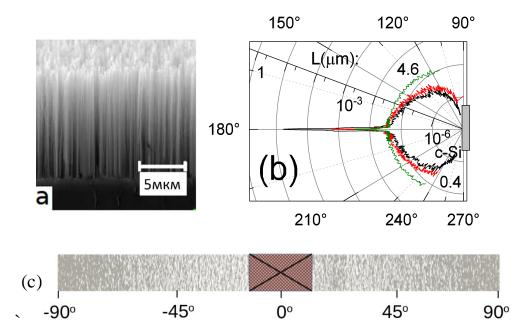
Fig 1s.4 (a) SEM image of silicon nanowires. (b) The cross section of the scattering indicatrix for the silicon c-Si and the silicon nanowires with lengths of 0.4 and 4.6  $\mu$ m under excitation at 1064 nm. (c) reconstruction of scattering panoramas in the backward hemisphere.
