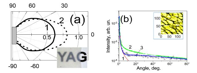
Fig 1s.2 a) Elastic optical scattering indicatrices of YAG laser ceramics with annealing temperatures of 400  $^{\circ}$ C (1) and 500  $^{\circ}$ C at 532 nm. The insert contains a photo of a sample of laser ceramics YAG. b) Comparison of different approximations for fitting of nanocrystalline silicon scattering indicatrices: 1) - RGD, 2) - amplitude-phase screen, 3) - T-matrix. The insert contains an AFM image of an nanostructured silicon film with thickness 10 nm.
