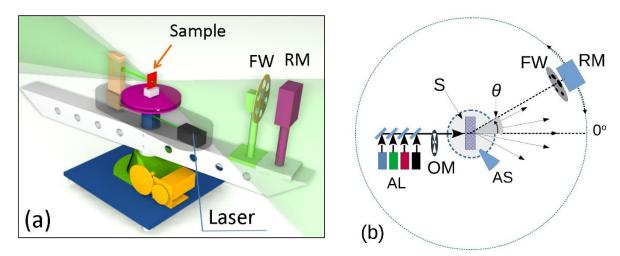
Fig. 2.1 a) Prototype of the instrument for measuring the cross-section of the elastic optical scattering indicatrix [65]. FW – wheel of neutral filters, RM – photodiode, photomultiplier, or CCD matrix (see appendix). b) Conceptual scheme of the setup: RM – registration module (PD, PMT, CCD), AS – angular position sensor, OM – optical modulator, AL – array of lasers (1064, 660, 532, 405 nm).
