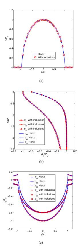
**Figure 3.6:** Validation of the enrichment technique with Hertzian analytical solution (a)  $_{66}$  Pressure distribution (b) Stresses along z direction (c) Stresses along y direction
