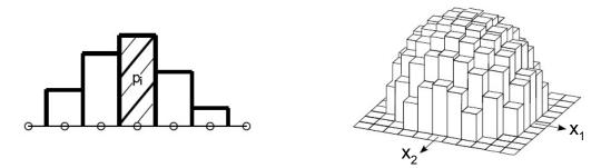
Figure 2.3: Discretizaton of the contact loading in  $N_p$  rectangles of uniform pressure and shears.
