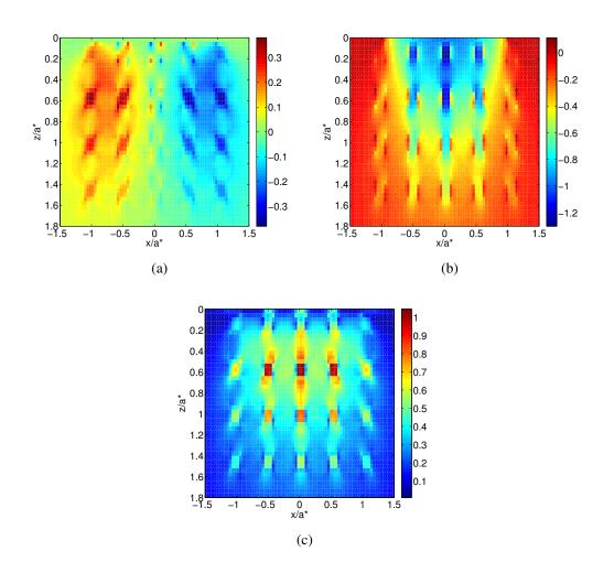
**Figure 6.9:** Dimensionless stress field (a)  $\sigma_{13}/P_0$  (b)  $\sigma_{33}/P_0$  (c)  $\sigma_{VM}/P_0$  in the plane y = 0 for a half space with a periodic structure of cuboidal inclusions ( $V_f = 0.1$ ).
