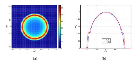
Figure 3.36: (a) Damage variable *D* with  $\mu = 0.7$  in the plane z = 0 in partial slip regime. (b) Contact pressure evolution with fretting cycles in the plane x = 0 using damage model from Ghosh et al. [GHO 13].
