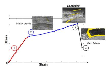
Figure 1.25: Behavior of a 3D woven composite in tension along the warp direction [HUR 14].
