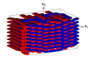
Yarns are modeled by placing ellipsoidal inclusions along the mean line of the yarn profile.
