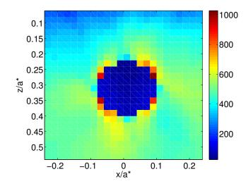
Figure 4.16: Delta shear stress  $\Delta \tau$  in MPa in the plane y = 0 with a very soft inclusion  $E_I = 10$ GPa.
