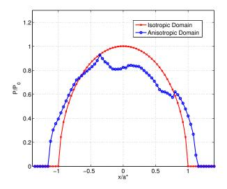
Figure 6.29: Contact pressure between the rigid cylinder and the isotropic domain and with the anisotropic domain.
