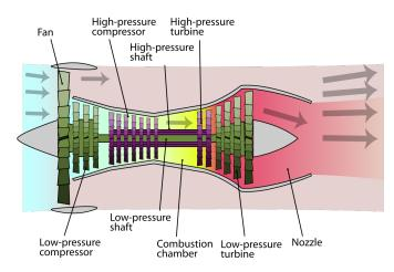
Figure 1.3: Schematic diagram of a high-bypass turbofan engine.
