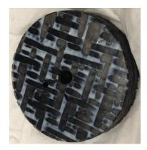
Figure 5.5: Disk made of woven composite material
