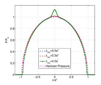
Figure 4.18: Comparison of the contact pressure with a spherical inclusion under the center of the contact for different inclusion's depth. Inclusion's diameter is  $d_{inc} = 0.16a^*$  and 1.5 times stiffer than the matrix ( $E_I/E_0 = 1.5$ ).
