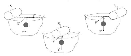
**Figure 4.7:** 3D view of the rolling of a cylinder on a elastic half-space with a spherical inclusion.
