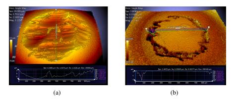
Figure 3.22: Wear scar of a steel ball (a) under gross slip regime (b) under stick-slip regime.
