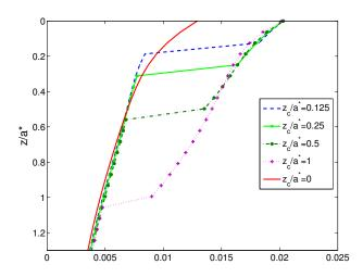
**Figure 3.30:** Equivalent strain along z for different thickness  $z_c$  and with a soft coating  $(\gamma = 0.5)$
