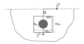
Figure 4.9: View of the REV around the spherical inclusion
