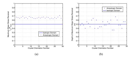
Figure 6.30: (a) Variation of magnitude in the maximum shear stress reversal in the 30 anisotropic domains. (b) Variation of the corresponding depth in the 30 anisotropic domains.
