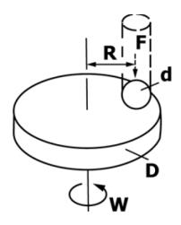
Figure 5.2: Description of Pin-on-Disk parameters
