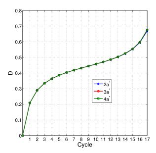
Figure 3.17: Effect of enrichment size on damage evolution
