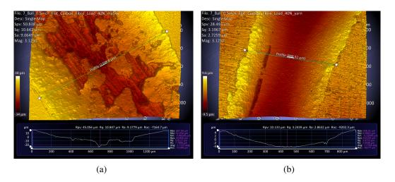
**Figure D.2:** N=5000 Cycles and W=40N (a) Contact surface on matrix. (b) Contact surface on yarn.
