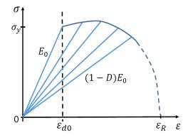
Figure 3.1: Stress-Strain plot with damage evolution.
