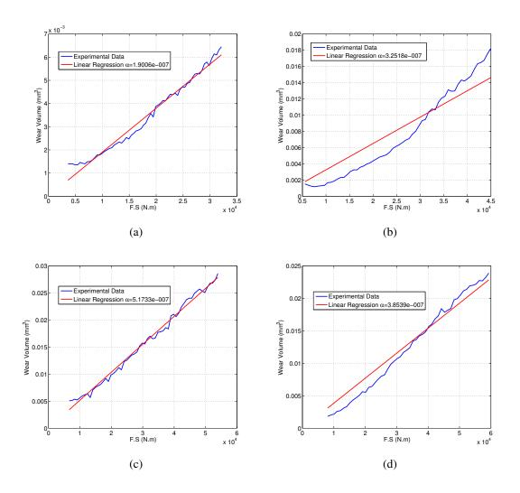
**Figure 5.8:** Wear Volume between AISI 52100 steel ball and composite disk function of the sliding distance and determination of the wear rate coefficient from a linear regression (α) for (a) 30 N (b) 50 N (c) 60 N (d) 80 N of normal load.
