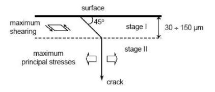
Figure 1.14: Crack initiation and propagation in partial slip fretting regime [FOR 61].
