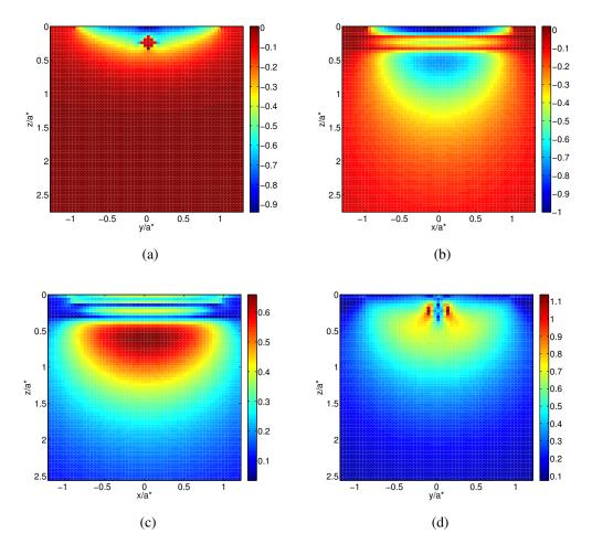
**Figure 6.20:** Dimensionless stress field in a unique yarn embedded into the matrix (a)  $\sigma_{11}/P_0$  in the plane x = 0 (b)  $\sigma_{33}/P_0$  in the plane y = 0 (c)  $\sigma_{VM}/P_0$  in the plane x = 0 (d) and y = 0.
