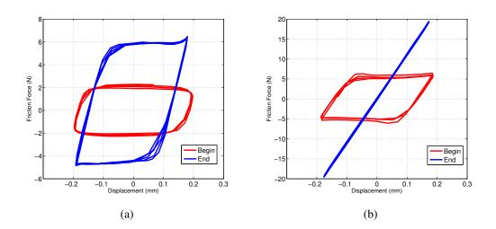
**Figure 5.13:** Fretting Loops at the beginning and end of the test after (a) W=20N on a yarn (b) W=30N on the matrix.
