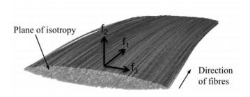
Figure 5.3: Transverse isotropy of yarn [NAO 15b].
