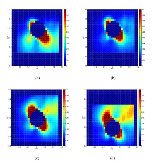
**Figure 4.14:** Damage variable D in the plane y = 0 with inclusion depth (a)  $z_{inc} = 0.3a^*$  (b)  $z_{inc} = 0.4a^*$  (c)  $z_{inc} = 0.5a^*$  (d)  $z_{inc} = 0.6a^*$ . The inclusion considered is 1.5 times stiffer than the matrix.
