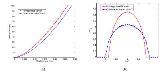
Figure 6.6: Comparison of the indentation curve (a) and of the dimensionless contact pressure with a normal load W = 100N (b) for a half space with one inclusion ( $V_f = 0.7$ ) in the REV and the corresponding homogenized domain.
