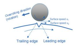
Figure 4.20: Definition of Over Rolling Direction [MOR 15]
