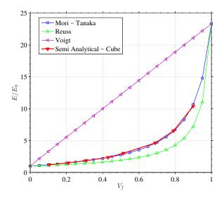
**Figure 6.5:** Effective Young modulus comparison with classic homogenization methods for one cuboidal inclusion embedded in a matrix with periodic boundary conditions. The Mori-Tanaka and the numerical technique curves match exactly.
