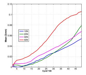
Figure D.5: In-situ wear depth between AISI 52100 steel ball and disk for different normal loads.
