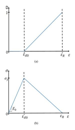
**Figure 3.2:** (a) Damage evolution as a function of strain showing the purely elastic domain and the damageable domain. (b) Purely elastic and damageable domains on a stress strain plot.
