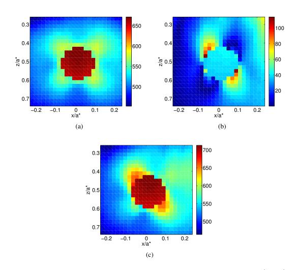
**Figure 4.10:** Alternating shear stress  $\tau_{alternating}$  (a), absolute mean shear stress  $|\tau_{mean}|$  (b) and their summation  $\Delta \tau$ (c) in MPa during one load pass over a half-space in the plane y = 0.
