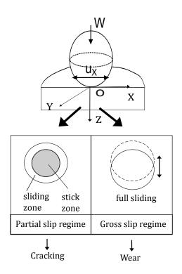
Figure 3.26: Fretting regime and associated damage phenomena
