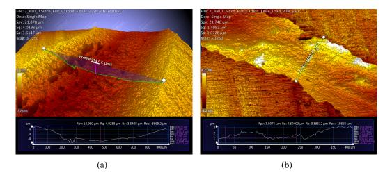
**Figure D.1:** N=5000 Cycles and W=20N (a) Contact surface on matrix. (b) Contact surface on yarn.
