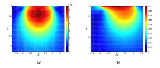
**Figure 3.8:** Equivalent strain  $\tilde{\varepsilon}$  (a) under normal loading in the plane x = 0. (b) under normal and tangential loading in the plane y = 0 with  $\mu = 0.5$  during the first fretting cycle.
