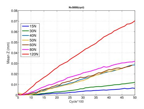
Figure 5.7: In-situ wear depth between AISI 52100 steel ball and woven composite disk for different normal loads.
