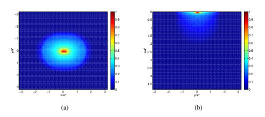
Figure 3.9: Damage variable *D* with  $\mu = 0.5$  (a) in the plane z = 0. (b) in the plane x = 0 after 17 cycles.
