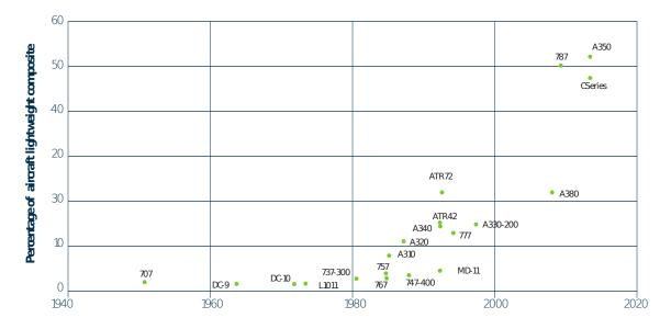
Figure 1.2: Growth in the use of composites in commercial aircraft [ATA 10].
