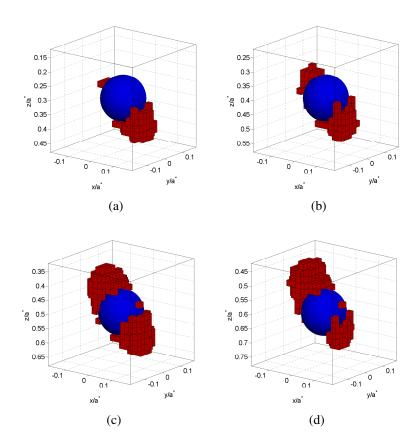
**Figure 4.15:** Butterfly wings around a spherical inclusion with inclusion depth (a)  $z_{inc} = 0.3a^*$  (b)  $z_{inc} = 0.4a^*$  (c)  $z_{inc} = 0.5a^*$  (d)  $z_{inc} = 0.6a^*$ . The inclusion considered is 1.5 times stiffer than the matrix.
