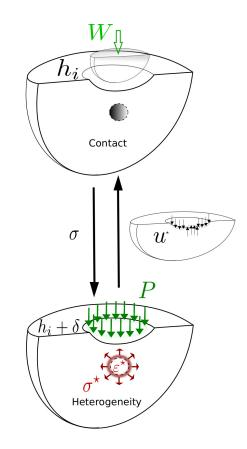
Figure 2.7: Iteration between contact problem and heterogeneous problem
