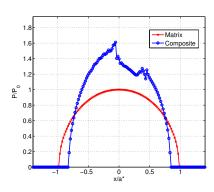
**Figure 6.18:** Contact pressure on the voxelized composite material (blue line) and on a homogeneous material with matrix elastic properties (red line).
