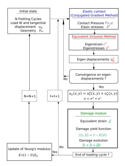
Figure 3.5: Algorithm of Heterogeneous Elastic-Damageable Contact Problem
