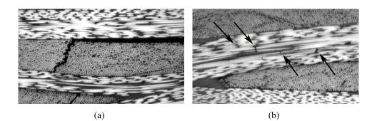
Figure 1.30: Damage of 2.5D-C/epoxy (a) Transverse crack and debonding of the yarn (b) Longitudinal crack of the yarn [COU 08].
