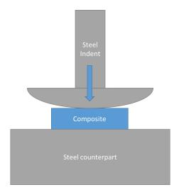
Figure 5.21: Schematic view of the compression experiment with MTS test rig.
