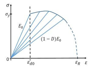
Figure 1.21: Stress strain curve with damage
