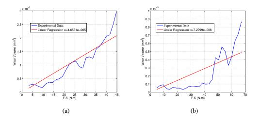
**Figure 5.20:** Fretting Wear Volume between AISI 52100 steel ball and the yarn of a composite material function of the sliding distance and determination of the wear rate coefficient from a linear regression ( $\alpha$ ) for a normal load equal to (a) 20 N (b) 30 N.
