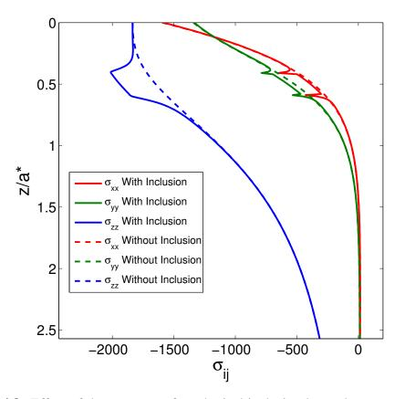
**Figure 4.8:** Effect of the presence of a spherical inclusion located at  $z_{inc} = 0.5a^*$  under the surface on the stresses at the center of the contact.Note that here the inclusion is 1.5 times harder than the matrix:  $E_I = 300GPa$ ,  $E_0 = 200GPa$ .
