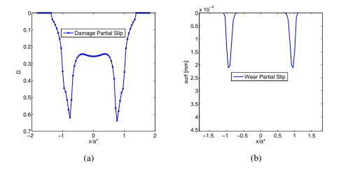
**Figure 3.41:** (a) Damage at the surface along *x* direction (b) Worn surface along *x* direction in the partial slip regime.
