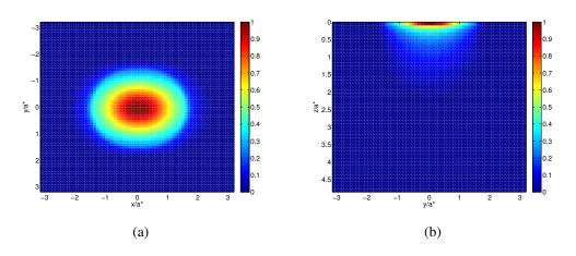
**Figure 3.13:** Damage variable *D* with  $\mu = 0.7$  (a) in the plane z = 0. (b) in the plane x = 0 after 4 cycles
