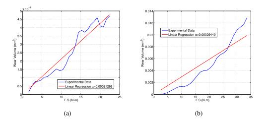
**Figure 5.19:** Fretting Wear Volume between AISI 52100 steel ball and the matrix of a composite material function of the sliding distance and determination of the wear rate coefficient from a linear regression ( $\alpha$ ) for a normal load equal to (a) 10 N (b) 15 N.
