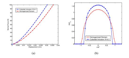
Figure 6.7: Comparison of the indentation curve (a) and of the dimensionless contact pressure  $P/P_0$  (b) for a half space with one inclusion ( $V_f = 0.1$ ) in the REV and the corresponding homogenized domain.
