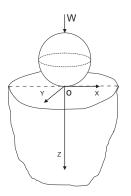
Figure 2.2: Contact of a sphere over an elastic half-space.
