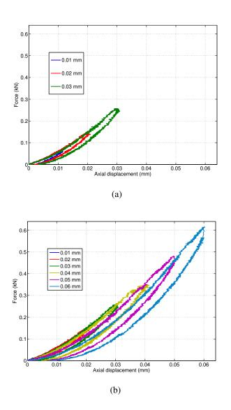
**Figure 5.23:** Force-Displacement curves of normal tests (a) from 0.01mm to 0.03mm of imposed axial displacement (b) Full cycle loading curves from 0.01mm to 0.06mm.
