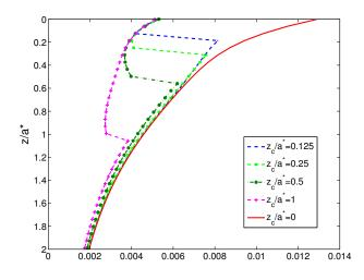
**Figure 3.31:** Equivalent strain along z for different thickness  $z_c$  and with a hard coating  $(\gamma = 2)$
