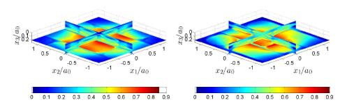
Figure 1.32: Von Mises stress during indentation of 2D composite material with semianalytical method [LER 13].
