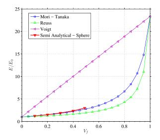
**Figure 6.4:** Effective Young modulus comparison with classic homogenization methods for one spherical inclusion embedded in a matrix with periodic boundary conditions. The Mori-Tanaka and the numerical technique curves match exactly.
