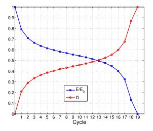
Figure 3.10: Evolution of damage and Young modulus with cycles for  $\mu = 0.5$
