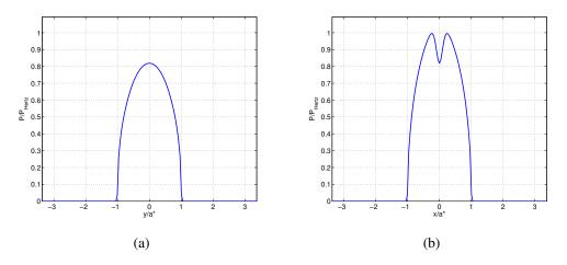
Figure 6.21: Contact pressure in the plane (a) x = 0 (b) y = 0.
