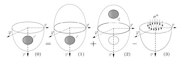
Figure 2.6: Decomposition of the half-space solution into three sub-problems
