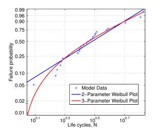
**Figure 6.35:** 2 and 3 parameters Weibull plot superimposed on the data from the model for the maximum Von Mises stress criterion.
