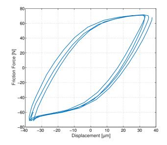
Figure D.8: Fretting Loop N=60000, W=125N and  $\delta=0.2mm$
