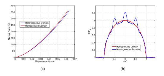
Figure 6.8: Comparison of the indentation curve (a) and of the dimensionless contact pressure  $P/P_0$  (b) for a half space with a periodic structure of cuboidal inclusions ( $V_f = 0.1$ ) and the corresponding homogenized domain.
