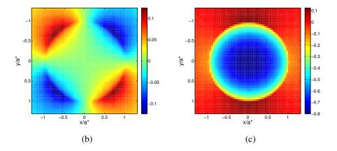
**Figure 6.14:** Dimensionless stress field in the plane z = 0 of a homogeneous material (a)  $\sigma_{11}$  (b)  $\sigma_{12}$  (c)  $\sigma_{22}$
