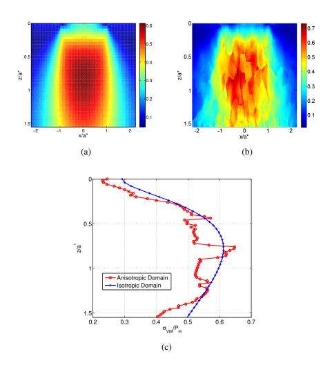
**Figure 6.28:** Dimensionless von Mises stress in the plane y = 0 (a) in an isotropic domain (b) in an anisotropic polycrystalline domain. (c) von Mises stress along z direction in the anisotropic domain and in the isotropic domain.
