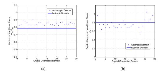
Figure 6.32: (a) Variation of magnitude in the maximum Von Mises stress in the 30 anisotropic domains. (b) Variation of the corresponding depth in the 30 anisotropic domains.
