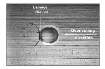
Figure 4.21: C-cracks around indent under rolling condition [MOR 15]
