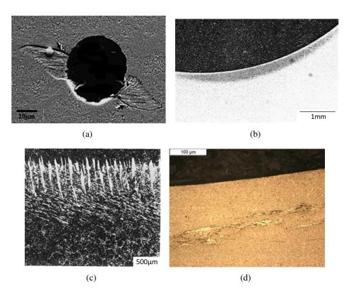
**Figure 1.19:** Damage mechanisms in Rolling Contact Fatigue (a) Butterfly wings around an inclusion [GRA 10] (b) Dark Etching Region in axial cross section (c) White Etching Flat and Steep Bands [ZWI 82] (d) White Etching Cracks in axial cross section [RUE 14].
