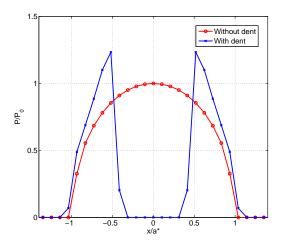
Figure 4.22: Contact pressure on the indented surface
