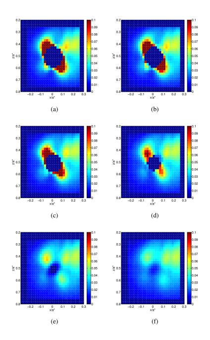
**Figure 4.12:** Sectioning of the damage variable D around an inclusion at  $z_{inc} = 0.5a^*$  in different planes parallel to the rolling direction. (a) Plane y=0 (b) Plane y=0.04 $a^*$  (c) Plane y=0.08 $a^*$  (d) Plane y=0.12 $a^*$  (e) Plane y=0.16 $a^*$  (f) Plane y=0.2 $a^*$ .
