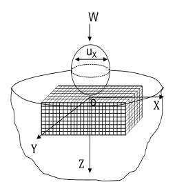
Figure 3.4: 3D view of a sphere on a elastic half-space with multiple cuboidal inclusions superimposition
