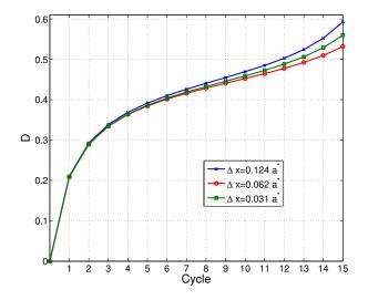
Figure 3.16: Effect of computation discretization on damage evolution
