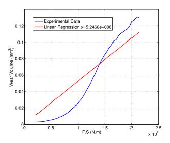
**Figure D.6:** Wear Volume between AISI 52100 steel ball and disk function of the sliding distance with W=40N. Obtention of the wear rate coefficient from a linear regression.
