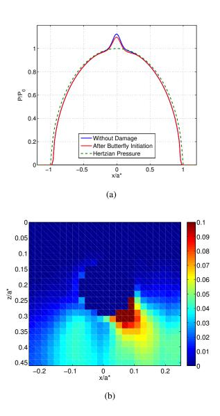
**Figure 4.19:** (a) Comparison of the contact pressure with a spherical inclusion of diameter  $d_{inc} = 0.16a^*$  and 1.5 times stiffer than the matrix ( $E_I = 300GPa$ ) under the center of the contact for a inclusion's depth  $z_{inc} = 0.2a^*$  before and after wing initiation. (b) Butterfly wing appearance in the plane y = 0.
