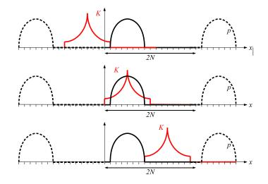
Figure C.2: Deleting overlapping using zero padding [GAL 07b]
