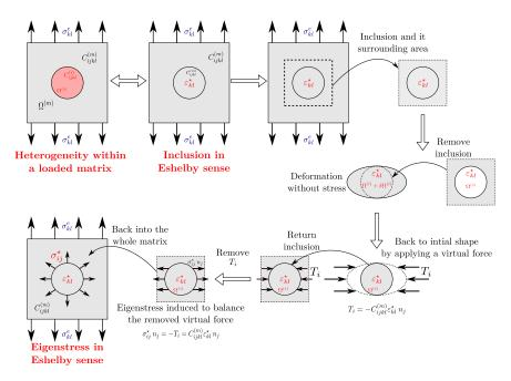
Figure 2.5: Single heterogeneity transformation into inclusion in the sense of Eshelby and subsequent eigenstress
