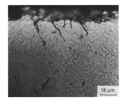
Figure 1.13: Crack initiation in partial slip fretting regime [BRY 88].
