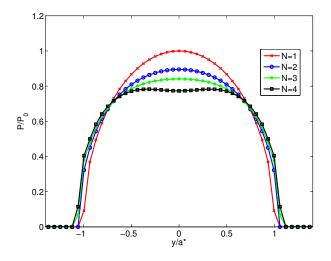
**Figure 3.14:** Effect of damage on contact pressure for  $\mu = 0.7$
