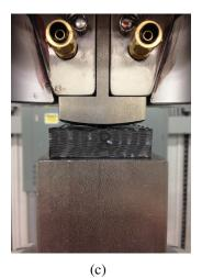
**Figure 5.22:** Normal test with MTS Engine (a) Indenter side view. (b) Indenter's tip view (c) View of experimental set up.
