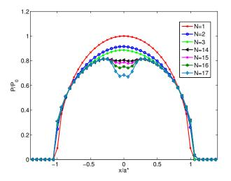
Figure 3.11: Effect of damage on contact pressure for  $\mu = 0.5$
