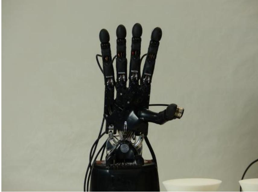
FIGURE B.1: Shadow Hand used in experiments.
