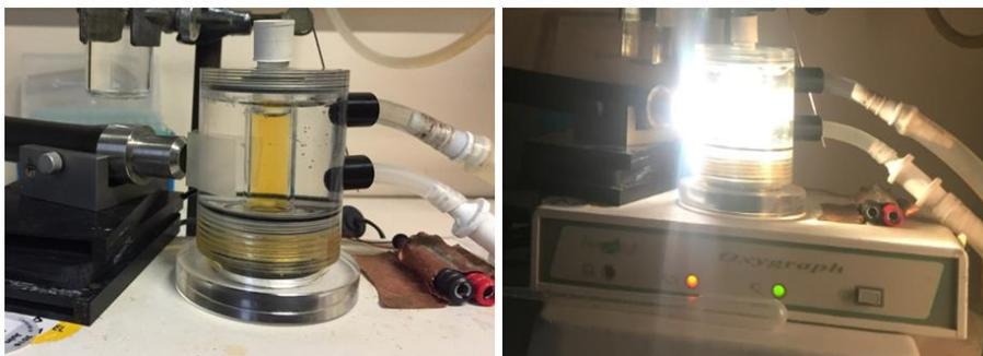
Figure 2-24 Experimental set-up : Clark Electrode before (left) and under illuminating (right)
