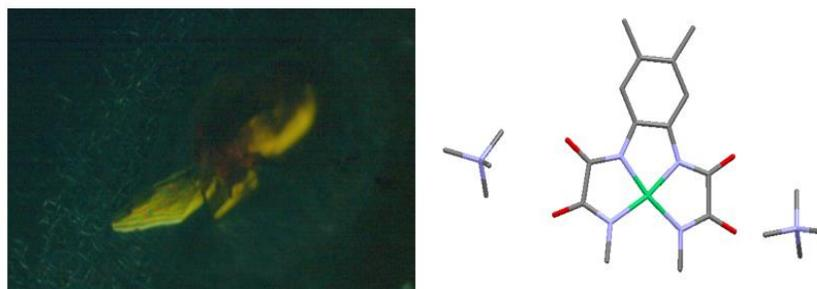
Figure C-2 Microscopic Crystal of Cu OPBI MV (left) and its structure (right).
