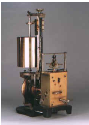
Figure 1.2. Kymographe vertical de Zimmermann (1907).
