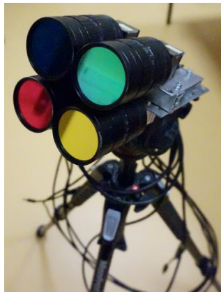
Figure F.1 Designed MS test sensor consisting of four identical IDS cameras equipped with 16 mm lens and four different filters {530, 63, 740, 810 nm} chosen for FD disease detection.
