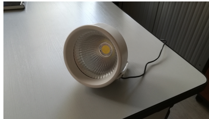
FIGURE 4.1: Photo of the phosphor-based white LED down-light used in the experimental setup.
