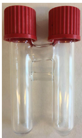
Figure 11. The sealed two-chamber system for the tandem reaction.
