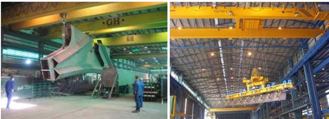
(a) Manipulating heavy part using multiple cranes (b) Crane with 10t vacuum prehension, 5 DOF
