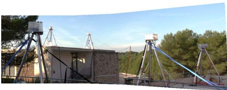
*Figure 1.8: The MARIONET crane prototype*
