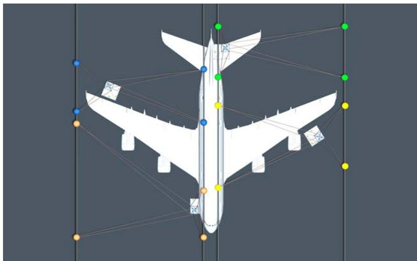
Figure 1.25: All pairs of winches can move on fixed rails along the airplane body
