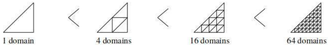
Figure B.7 – Here is shown one mesh refinement, for a mesh made of 1 domain to a mesh mdoe of 64 domain. Usually, the finer the mesh is, the better the solution will be.
