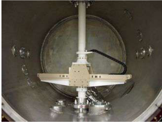
(c) The mapper in the nEDM vacuum tank.
