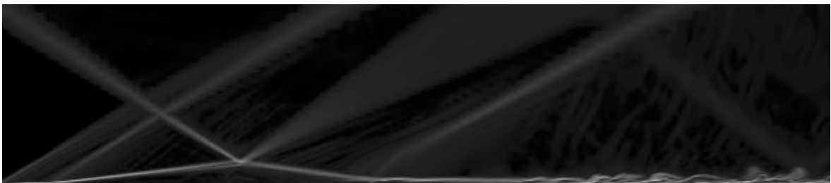
FIGURE 4.2 – Numerical schlieren visualization obtained by plotting the isocontours of the magnitude of the density gradient |\nabla\rho| (2D slice located at the middle of the domain).
