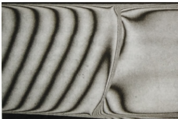
FIGURE 1.4 – Schlieren visualization of a normal shock wave from Babinsky and Harvey [2011].
