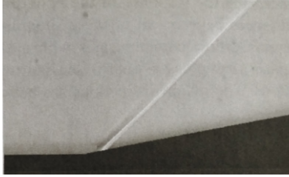
FIGURE 1.2 – Schlieren visualization of a ramp induced shock wave from Babinsky and Harvey [2011].
