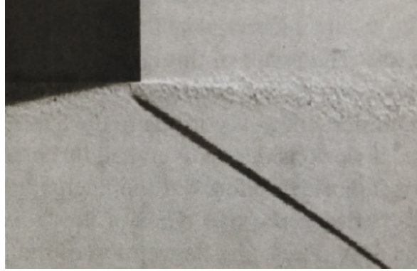
FIGURE 1.5 – Schlieren visualization of an adaptation shock wave at an overexpanded nozzle exit from Babinsky and Harvey [2011] .
