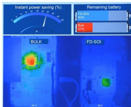
Figure 2-12. Temperature of UTBB vs Bulk [20]
