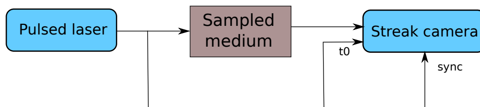
Figure 2.9: Standard setup for time-resolved systems based on streak cameras.
