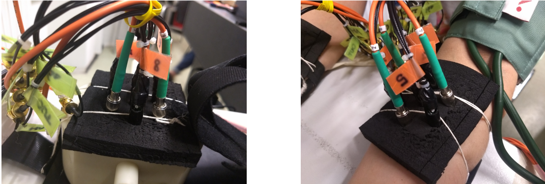
Figure 5.8: (Left) One of the probes located at the surface of a solid switchable phantom. (Right) Probe located at the arm of one of the subjects during arm occlusion experiment. Green and black probes are sources and detectors respectively.
