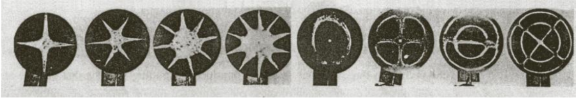
Figure 1.1: Cladni patterns on vibrating circular plates, from [42].
