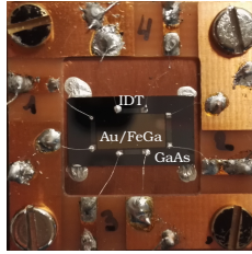
Figure 4.13: Chamber, used for the acoustic measurements.
