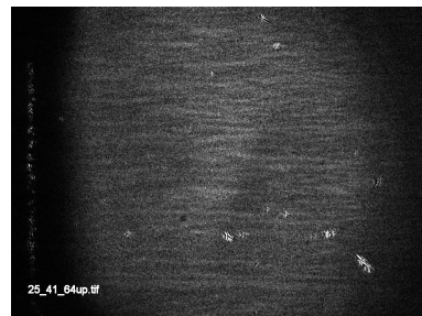
Figure 5.19: Kerr microscopy image taken at 4.2 mT, increasing field, \angle(\vec{B}, \vec{k}_{saw}) = -5^\circ
