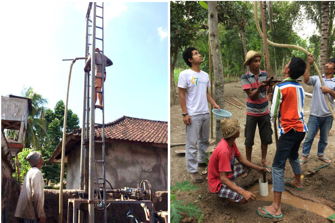
Figure 32. New cores drilling were conducted in the research area using the material and expertise of local drillers (Courtesy: B. Septiangga, July 2017).
