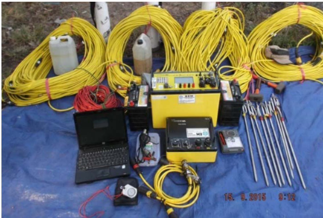
Figure 34. Geophysical measurements using a resistivity meter namely SuperSting (Courtesy: Y. Sudrajat, September 2015).
