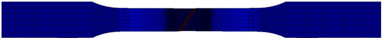
Fig. IX-4 Distributions of final fracture obtained from the local damage model for different mesh sizes
