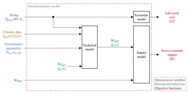
Figure IV-11 – Block diagram considered for investigating the influence of the error in the demand model output.
