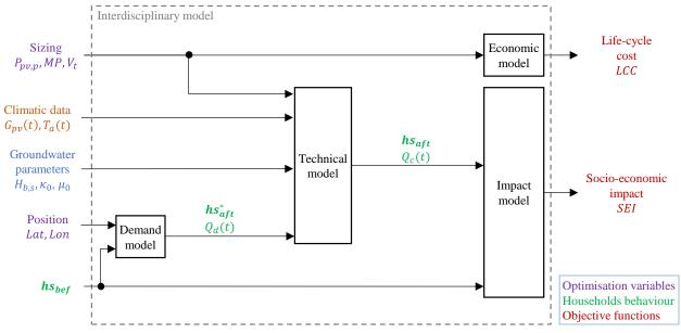
Figure III-1 – Block diagram of the interdisciplinary model.
