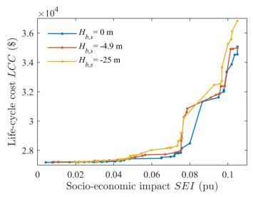
Figure IV-14 – Pareto fronts obtained for different values of the static water level H<sub>b.s</sub>.
