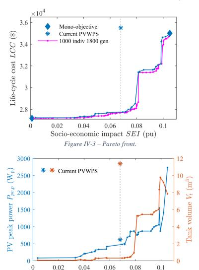
Figure IV-4 – Variation of  $P_{pv,p}$  and  $V_t$  as a function of the SEI.
