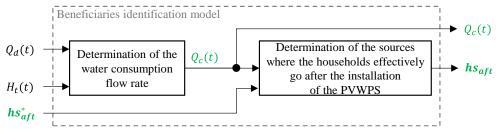
Figure III-17 – Block diagram of the beneficiaries identification model.
