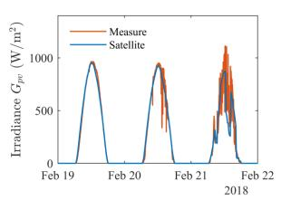
Figure C-2 – Comparison of the irradiance on the plane of the PV array from local measurements and from satellite data.
