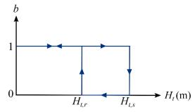
Figure III-8 – Controller model.
