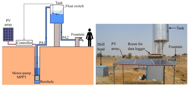
Figure II-7 – Architecture of the PVWPS.
