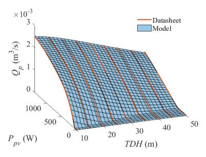
Figure III-9 – Model of the motor-pump SQFlex 5A-7.
