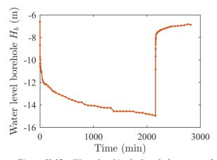
Figure II-12 – Water level in the borehole measured during the long pumping test (pump flow rate: 1.8 10<sup>-3</sup> m³/s).
