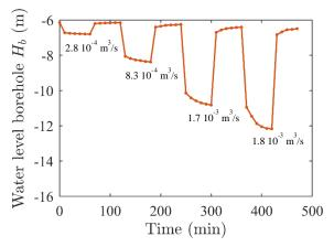
Figure II-11 – Water level in the borehole measured during the step pumping tests.
