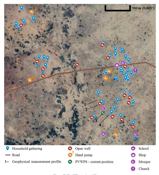
$\label{eq:figure II-10-GIS mapping of Gogma.} Data\ collected\ between\ the\ 18\ September\ 2017\ and\ the\ 10\ November\ 2017.$
