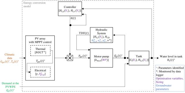
Figure III-6 – Block diagram of the energy conversion model.
