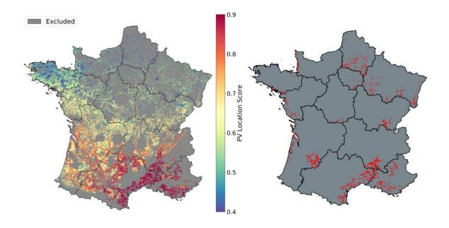
Figure 54: PV installation placement considering the multi-criteria approach
