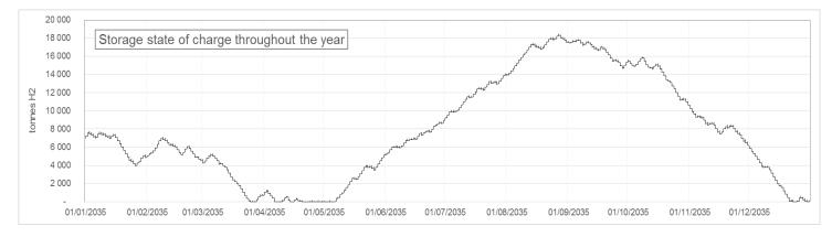
Figure 79: Hydrogen storage needs for the 5% penetration rate scenario
