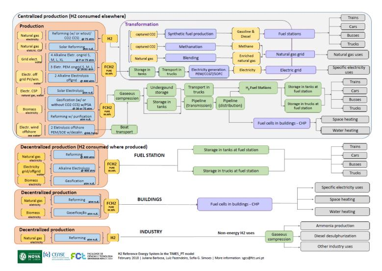
Figure 37: Hydrogen modelling structure in TIMES-PT
