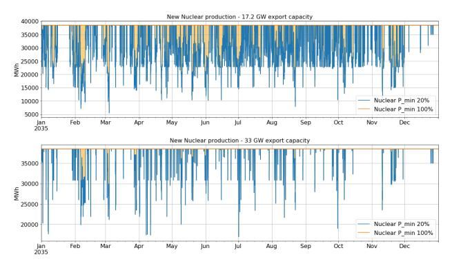
Figure 67: Nuclear generation profile and available energy for the two alternatives of export capacity. The upper figure corresponds to the 17.2 GW export capacity case study and the lower figure to 33 GW one
