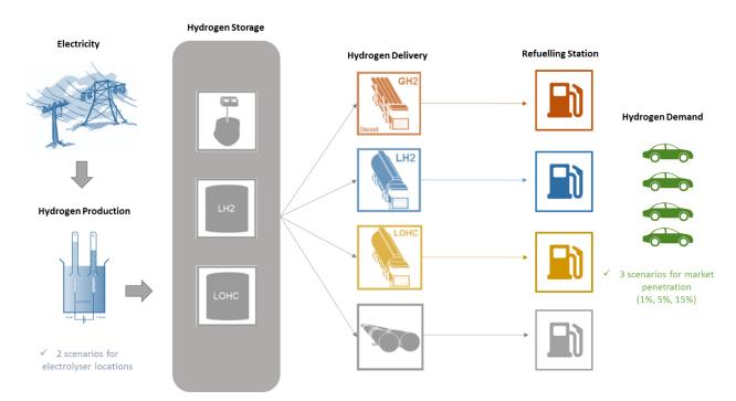
\*GH2: Gaseous hydrogen - LH2: Liquid hydrogen - LOHC: liquid organic hydrogen carrier Figure 72: Representation of the considered hydrogen supply chains
