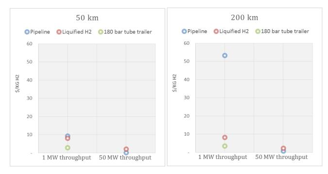
Figure 29: Hydrogen transport pathways comparison (adapted from [14])
