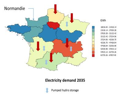
Figure 60: Electricity demand distribution by region (blue arrows show the locations of pumped hydro storage facilities; red arrows point to the five regions with the highest installed power generation capacities).
