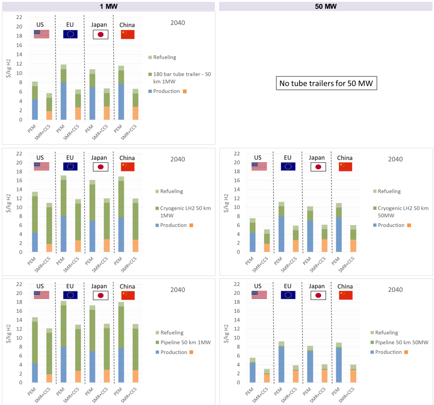
Figure 32: Hydrogen cost at the pump for the centralized case study in 2040 (left column 1 MW, right column 50 MW of throughput capacity, each line corresponds to a delivery pathway)
