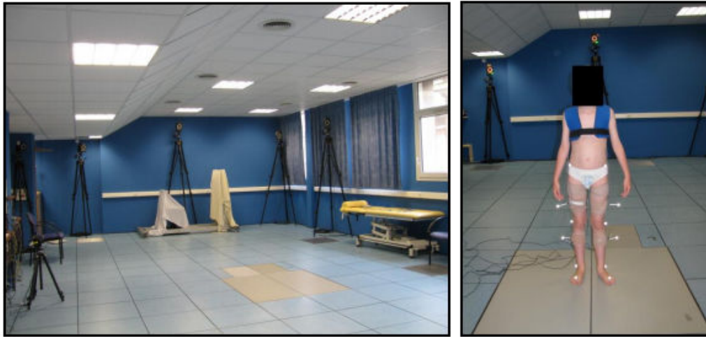
Figure 1.4: Motion analysis laboratory at the CHRU Morvan and an example of a typical set-up for reflective marker placements on a healthy child.
