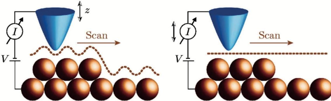
Figure 2.5: The STM imaging modes [36]: (left) constant-current mode, (right) constant-height mode.
