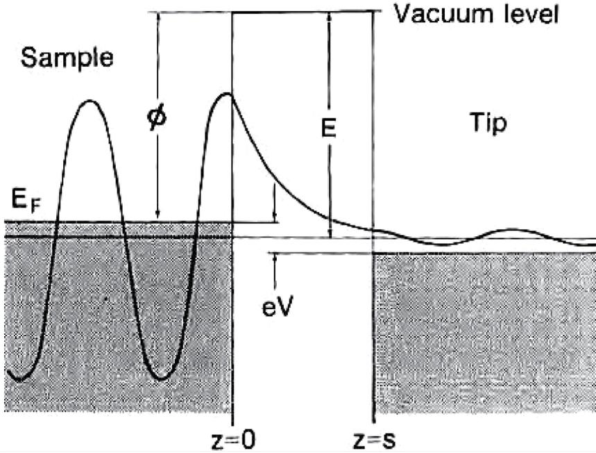
Figure 2.6: Schematic diagram of metal-vacuum-metal tunnelling [35]. Metals are indicated by the grey shadowing and represent the metal sample (left) and the tip (right). The middle region corresponds to the vacuum.
