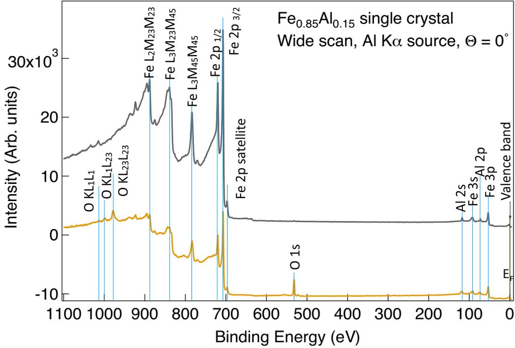
Figure 2.10: Al-K $\alpha$  wide scan of a clean and oxidised  $\text{Fe}_{0.85}\text{Al}_{0.15}$  where the main photoemission core levels and Auger transitions are pointed. Notice the increase of background at low kinetic energy due to inelastic electrons.
