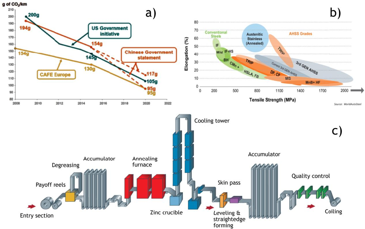
Figure 1.1: a) Worldwide convergence of objectives for CO<sub>2</sub> emission of cars per km [2]. b) Global formability diagram for today's Advanced High-Strength Steel grades including a comparison to traditional low-strength and high-strength steels [1]. c) Scheme of the industrial process of hot-dip galvanization of steel sheets [3].
