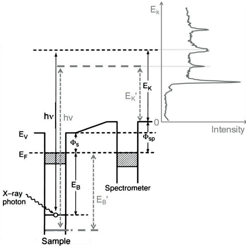
Figure 2.8: Link between schematic band level alignment between sample and spectrometer and photoemission spectrum in kinetic energy.  $\Phi_s$  is the work function of the sample *i.e.* the minimum energy required to extract an electron from the Fermi level to infinity [49].
