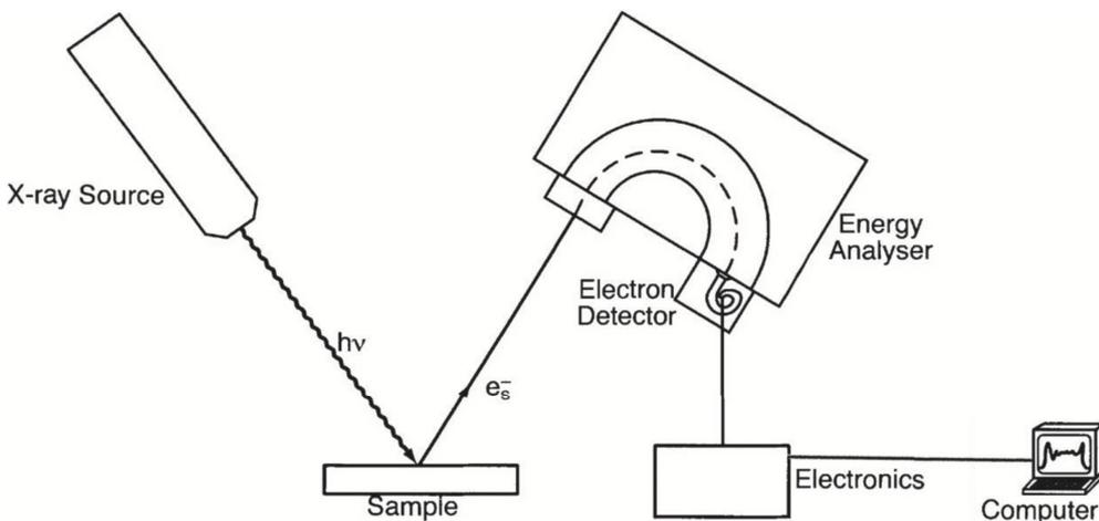
Figure 2.9: Main components for a typical XPS apparatus [48].
