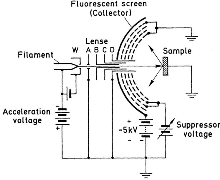
Figure 2.2: Schematic of a four-grids LEED optics.
