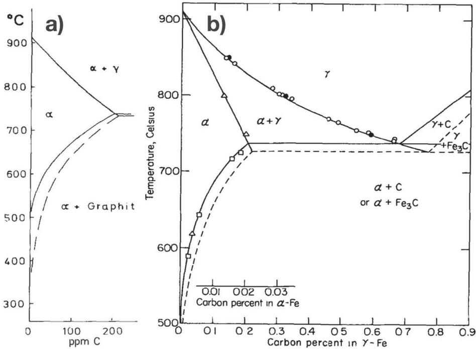
Figure 4.3: a) Carbon solubility at low-carbon concentration in the  $\alpha$  (bcc) phase of the C-Fe binary phase diagram [222]; b) C-Fe phase diagram where the dashed lines indicates the metastable Fe- $\text{Fe}_3\text{C}$  system [232].
