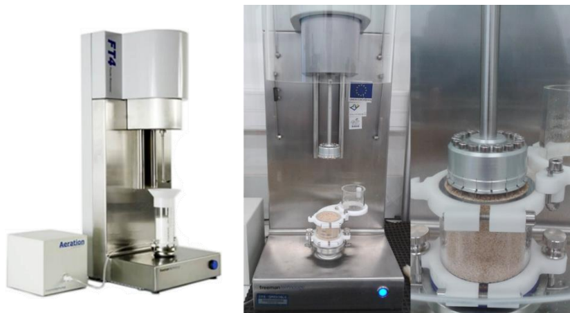
Figure 23: From left to right: FT4; shear cell in high position; Shear cell in rotation
