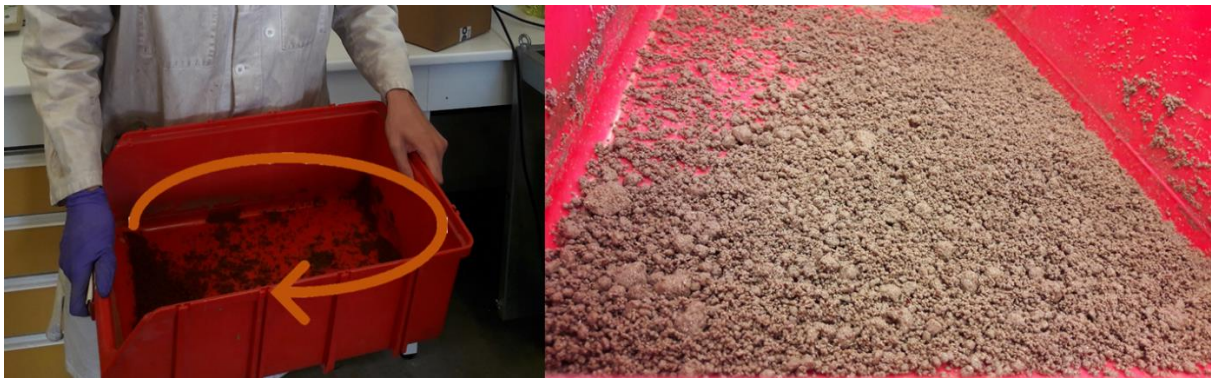
Figure 53: Granulation method. On the left, mixture in the tray being agitated. On the right, wet granulated mixture.
