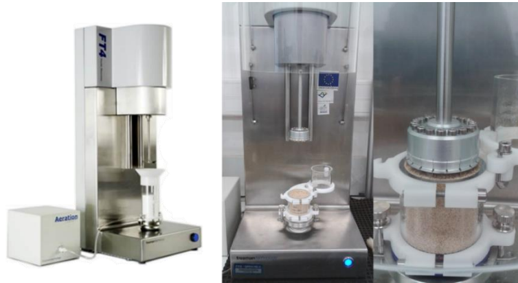
Figure 41: From left to right: FT4; shear cell in high position; Shear cell in rotation
