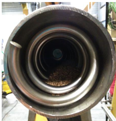
Figure 86: Left, picture of the shaftless screw feeder (axial view). Right, section of the reactor showing the bottom part of the injection system (side view).
