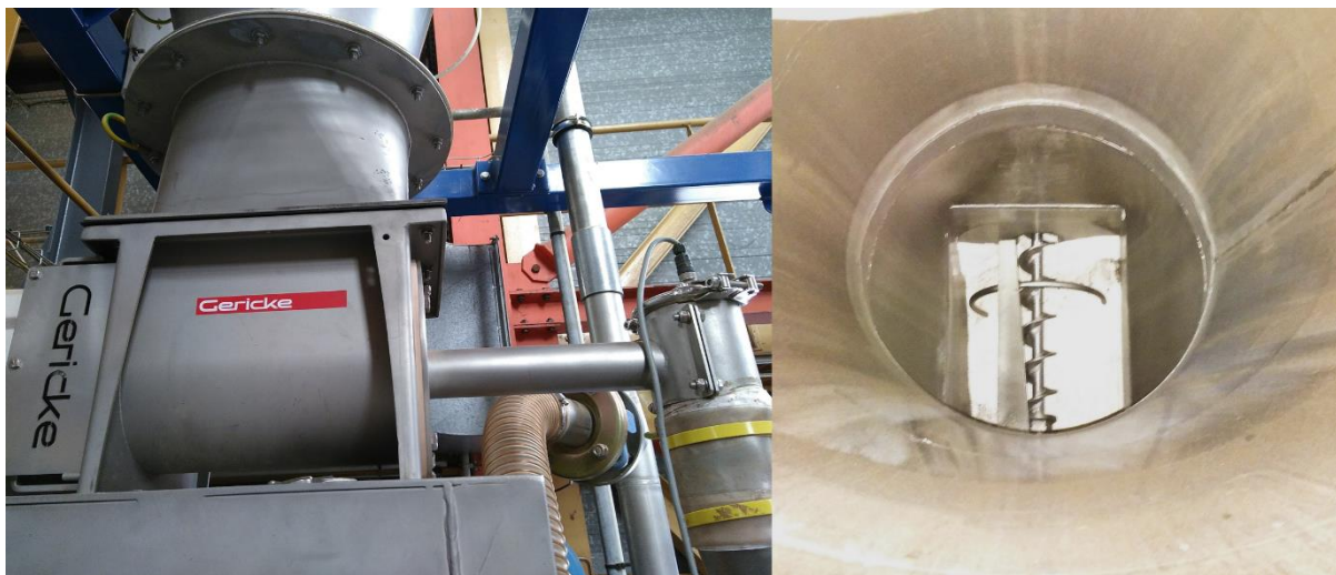
Figure 91: Left, picture of the screw in its opaque casing. Right, picture of the screw and the anti-bridging system from the top of the empty feeding hopper.
