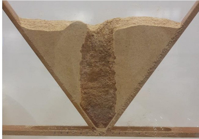
Figure 2: Ratholing during the discharge of a hopper with a wood powder.
