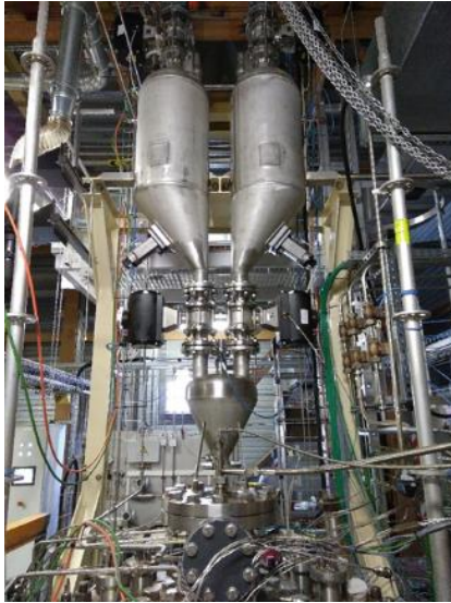
Figure 83: Injection system of the gasifier. Left, schematic of the whole injection system (lock-hoppers and screw feeder). Right, screw feeder, injection cone and injection tube.
