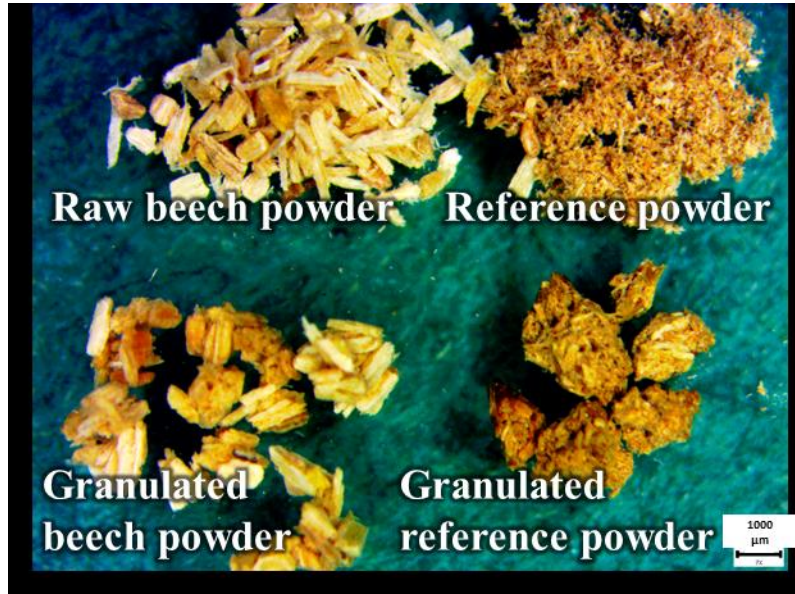
Figure 108: Picture of raw and granulated powders, observed with a 7x binocular magnifier.
