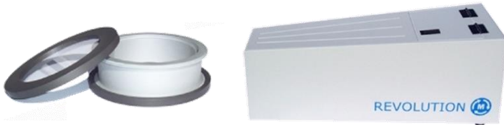
Figure 45: Left, drum containing the powder, to be placed in the analyzer. Right, Revolution powder analyzer [32]
