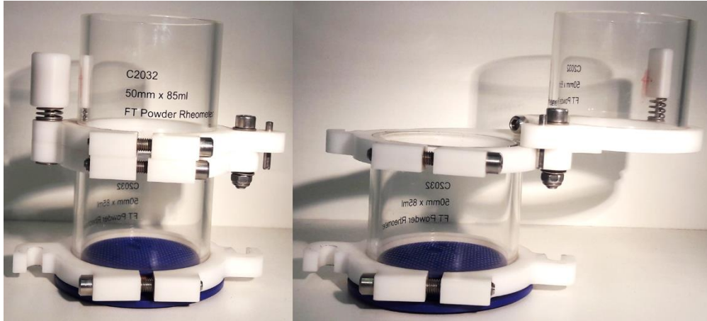
Figure 43: split vessel. Left, before splitting. Right, after splitting.
