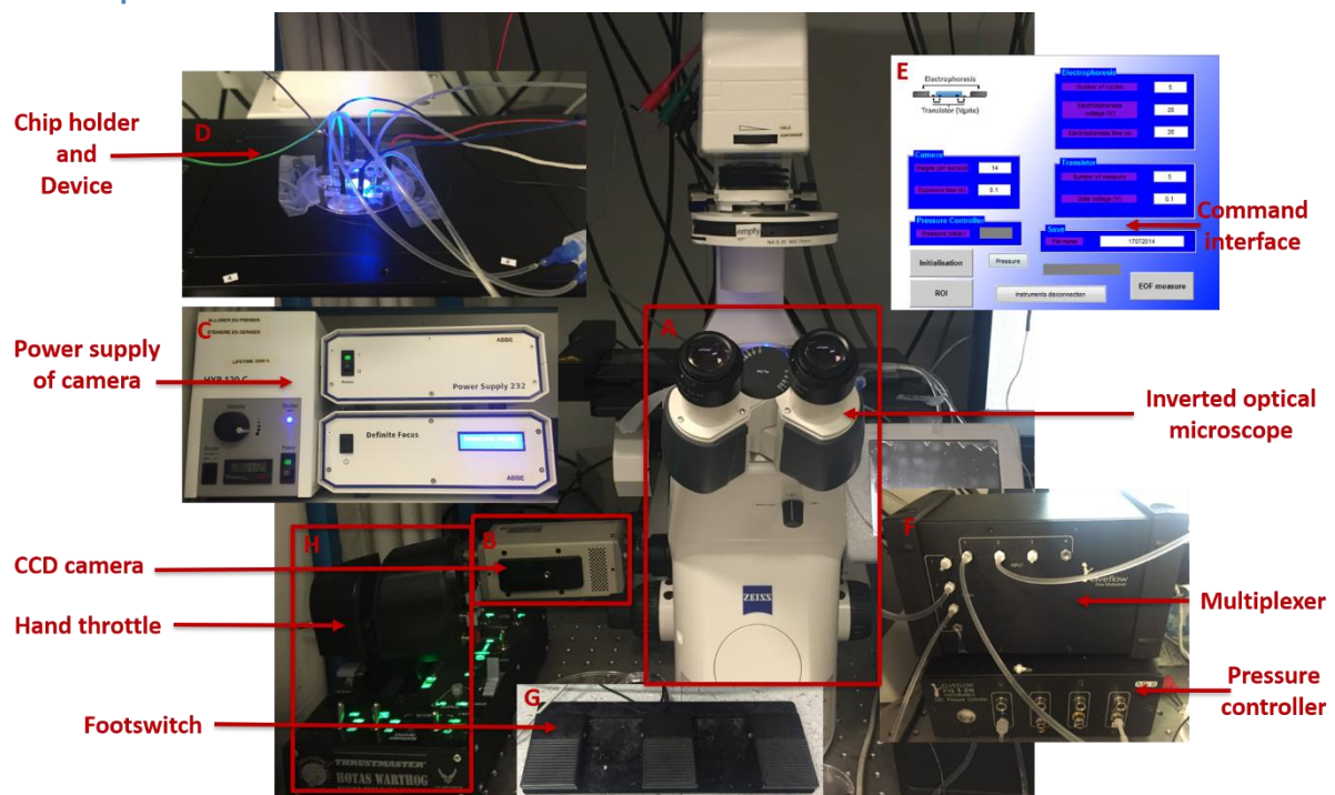
Figure 3.7: Total view photographs of the experimental bench. (A)- Inverted optical microscope. (B, C)- CCD camera and its power supply. (D)- Chip holder. (E)- Matlab® command interface. (F)- Fluid multiplexer and pressure controller. (G, H)- Footswitch and hand throttle.
