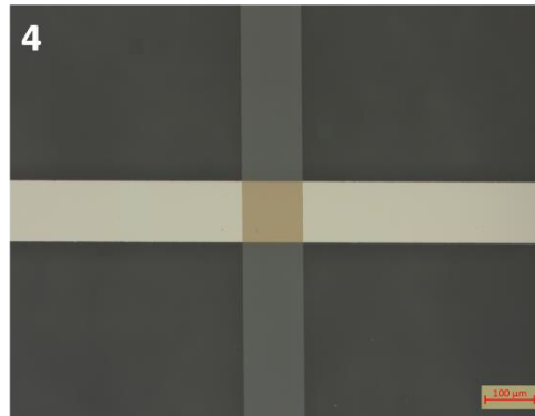
Figure 4.20: Top view of the fabrication processes of the cross thin layered Sample 3. 1- The cleaning process. 2- The 5/25 nm Ti/Pt physical vapor deposition. 3- The 20 nm CNx sputtering deposition. 4- Optical micrograph of the fabricated device.
