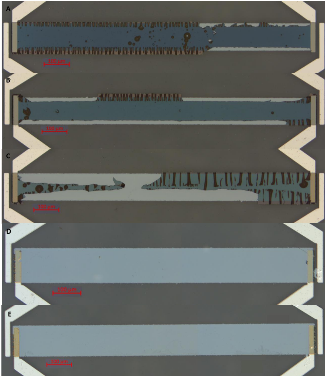
Figure 4.14: Top view micrographs of CNx polarizable films with different RF magnetron sputtering deposition conditions. (A)- 200W of power and 0.4 Pa of gas pressure. (B)- 220W and 0.4 Pa. (C)- 240W and 0.4 Pa. (D)- 200W and 0.6 Pa. (E)- 200W and 0.8 Pa. Noted that all the samples were immersed in the same 10^{-3}\text{M} KCl solution at clean-room temperature for four days.
