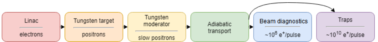
Figure 3.1: General scheme of the slow positron production line.
