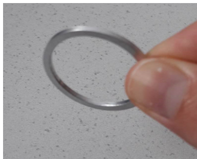
Figure B.6: Metal ring used to increase the MCP/CCD detector resolution.
