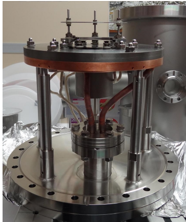
(a) Tungsten target together with the water cooling system.
