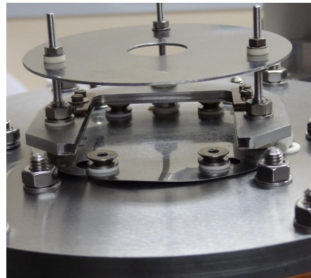
(b) Tungsten target with the support for the tungsten mesh and the accelerating electrode.
