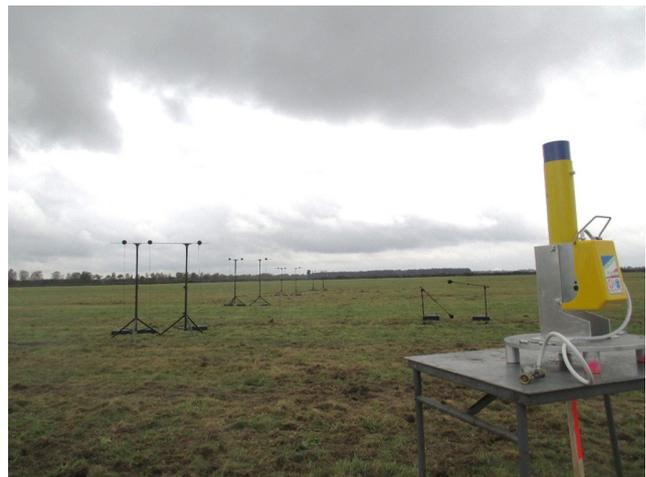
FIG. 1. (Color online) Measurement apparatus, with the gas cannon (on the table), two separate acoustic modules (on the right), and the four 3-modules bars at ranges 10, 20, 35, and 50 m (on the left). The microphones with foam wind screens are located on horizontal bars. The recording system of each module is in a small case on the ground.
