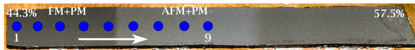
Figure 3.33. Ellipsometry measurements were made across an annealed Fe_{1-x}(Rh-Pt)_x strip, from the FM side to the AFM side. The measured points are illustrated with blue circles in this image. The composition shown on this figure is the (Rh + Pt) content.
