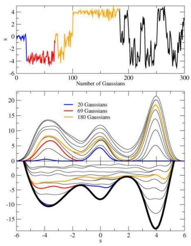
Figure 9: This figure was reproduced from[56] and it provides a typical example of a converged metadynamics simulation. The upper panel plots the CV value  $(s_{\alpha}(t))$  vs. the number of Gaussians added. The middle panel represents the evolution of the bias potential V(s,t) when increasing the number of Gaussians. The lower panel is the evolution of the sum of V(s,t) and  $\tilde{F}(s)$ , estimate of the free energy which is depicted by the thick black line.
