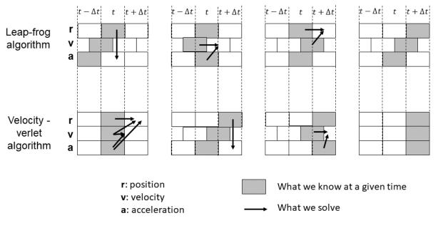
Figure 4: Schematic explanation of the propagations of the motions based on two algorithms: leap-frog and velocity-verlet algorithms
