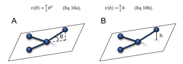
Figure 3: Representation of the out-of-plane torsions adapted from Molecular Modelling. Principles and Applications, by A.R. Leach, 2001.
