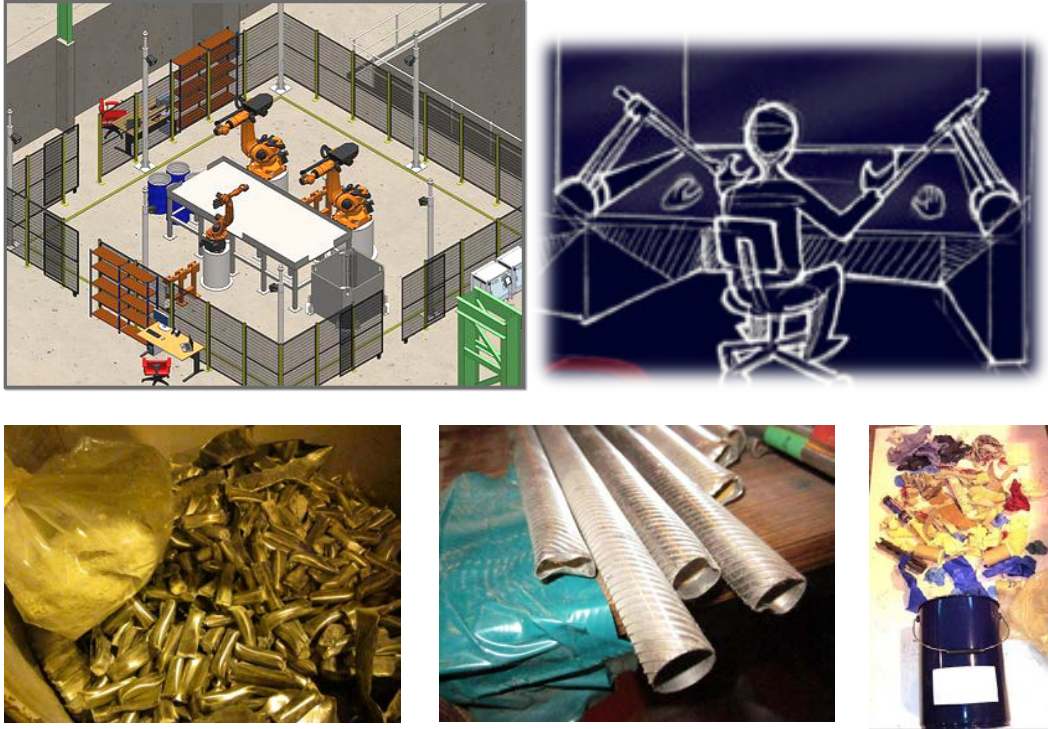
Figure 3.1: Top figures: an illustrative sketch of the robotic testbed envisioned for the RoMaNS sort and segregation tasks (left) with a human operator in partial control of the overall motion (right). Bottom figures: examples of the typical waste material to be handled by the robotic cell.
