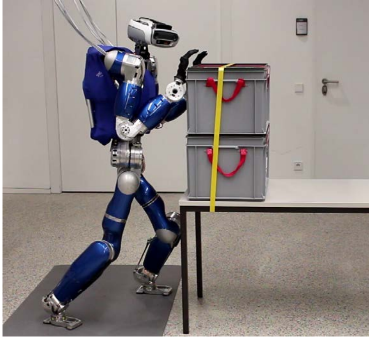
Figure 7.1: TORO pushing a table with a weight of 50 kg on top.
