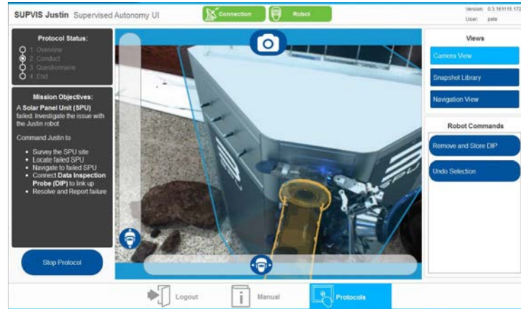
Figure 2.4: The tablet interface used in the SUPVIS Justin experiment. A rich graphical interface with augmented reality overlays allow for an easy and user-friendly experience of supervisory teleoperation. Photo courtesy [83].
