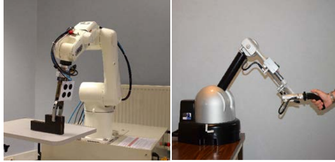
Figure 5.1: Left: the slave manipulator arm. The object to be manipulated is on the table in front of the slave robot. Right: The master device used by the operator for sending commands to the slave manipulator and receiving force cues.
