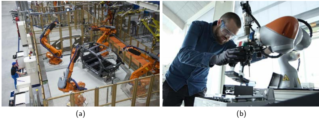
Figure 2.1: (a) Position/Velocity controlled manipulators placed in a cage and tele-operated by a human operator. Photo courtesy [38]. (b) A human operator interacting physically with a lightweight robot. Photo courtesy [39].
