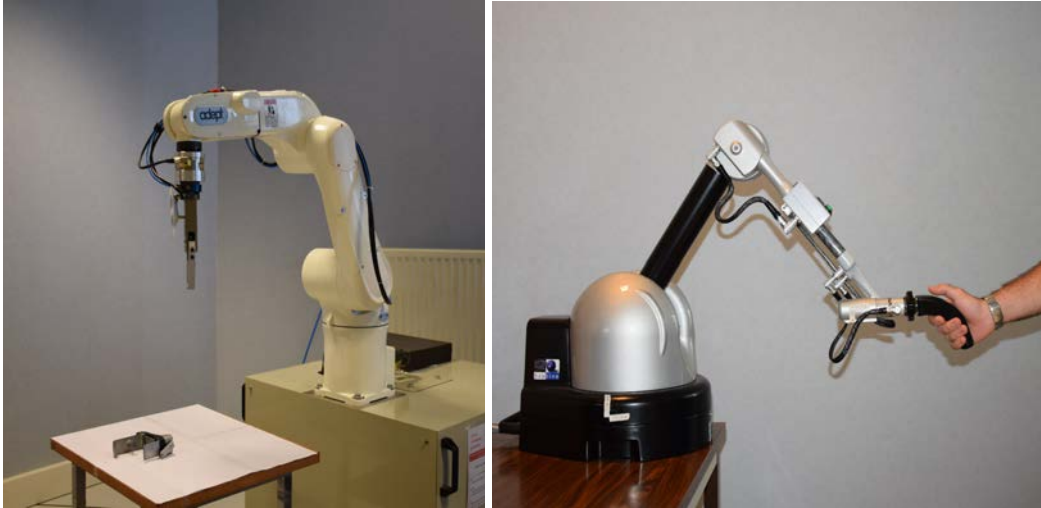
Figure 4.14: The experimental setup showing the slave robotic arm on the left and the master haptic arm on the right.
