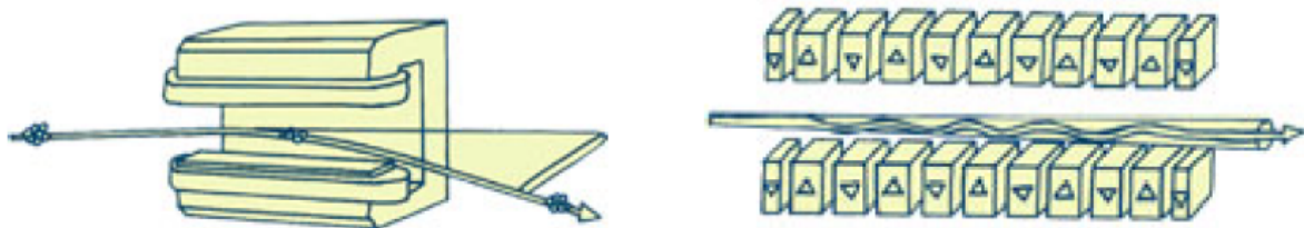
Figure 11: Bending magnet(left) and insertion device(right)
