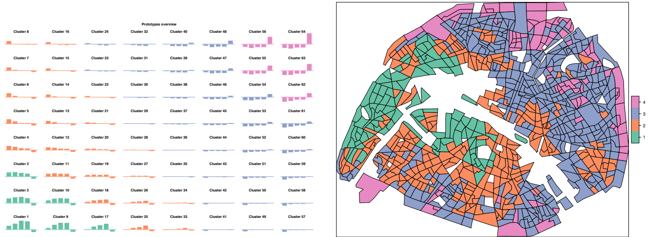
Figure 5.1: Left: the Kohonen map for the variables of Set 1, with values of the variables for the prototypes in each cluster. Colors indicate the final super-clusters obtained with HAC. Right: Spatial distribution of the four super-clusters obtained with the variables of Set 1. Areas in white correspond to parks, train stations, hospitals, and blocks for which data is not available.
