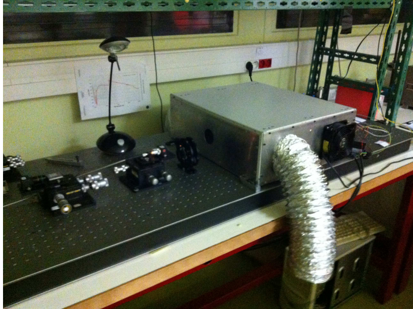
Figure 4.8: Optical setup for supercontinuum.
