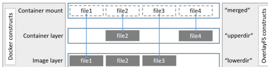
Figure 3.6 – Docker union file system: overlayfs [4]
