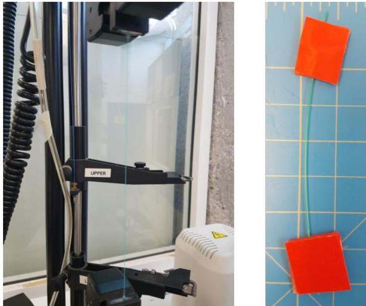
Figure 6.22: Left: Internal catheter sample undergoing tensile tension test in the Instron 3365 universal material testing machine. Right: Section of the internal catheter with double sided tape to help grip the sample.
