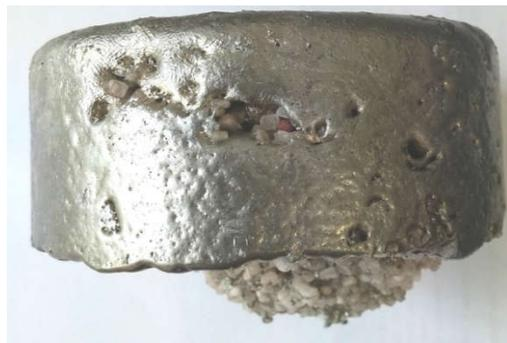
Fig. 2.13. Defects in the sample generated in injecting process
