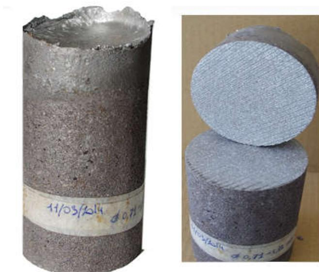
Fig. 2.26. Photos of the sample with a riser
