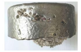
Fig. 2.13. Defects in the sample generated in injecting process
