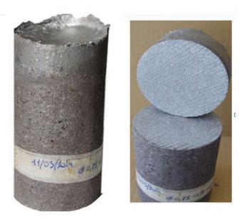
Fig. 2.26. Photos of the sample with a riser
