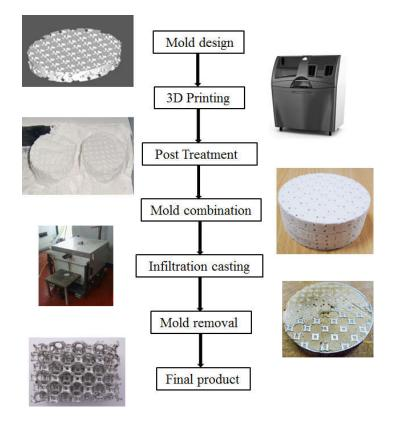
Fig. 5.20. Manufacturing process of aluminum foam with modified structure
