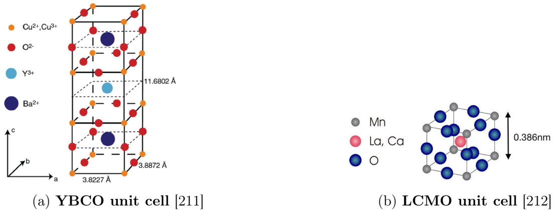
Figure 3.2: Unit cells of YBCO and LCMO
