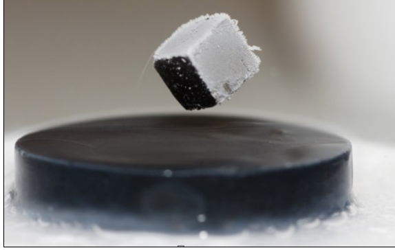
Figure 1.1: Magnetic levitation in cuprate \text{YBa}_2\text{Cu}_3\text{O}_7 Below its critical temperature, the superconducting cylinder repels magnetic fields. A small magnet placed above floats due to diamagnetism.
