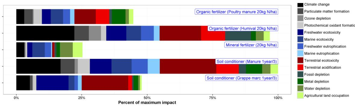
**Figure 11 : Comparison of environmental impact of 5 different alternatives for fertilisation for TMR1\_S2.**
