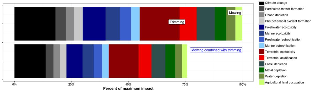
**Figure 13 : Comparison of environmental impacts of two unit operations with their combination in a unique operation for TMR2\_S2**
