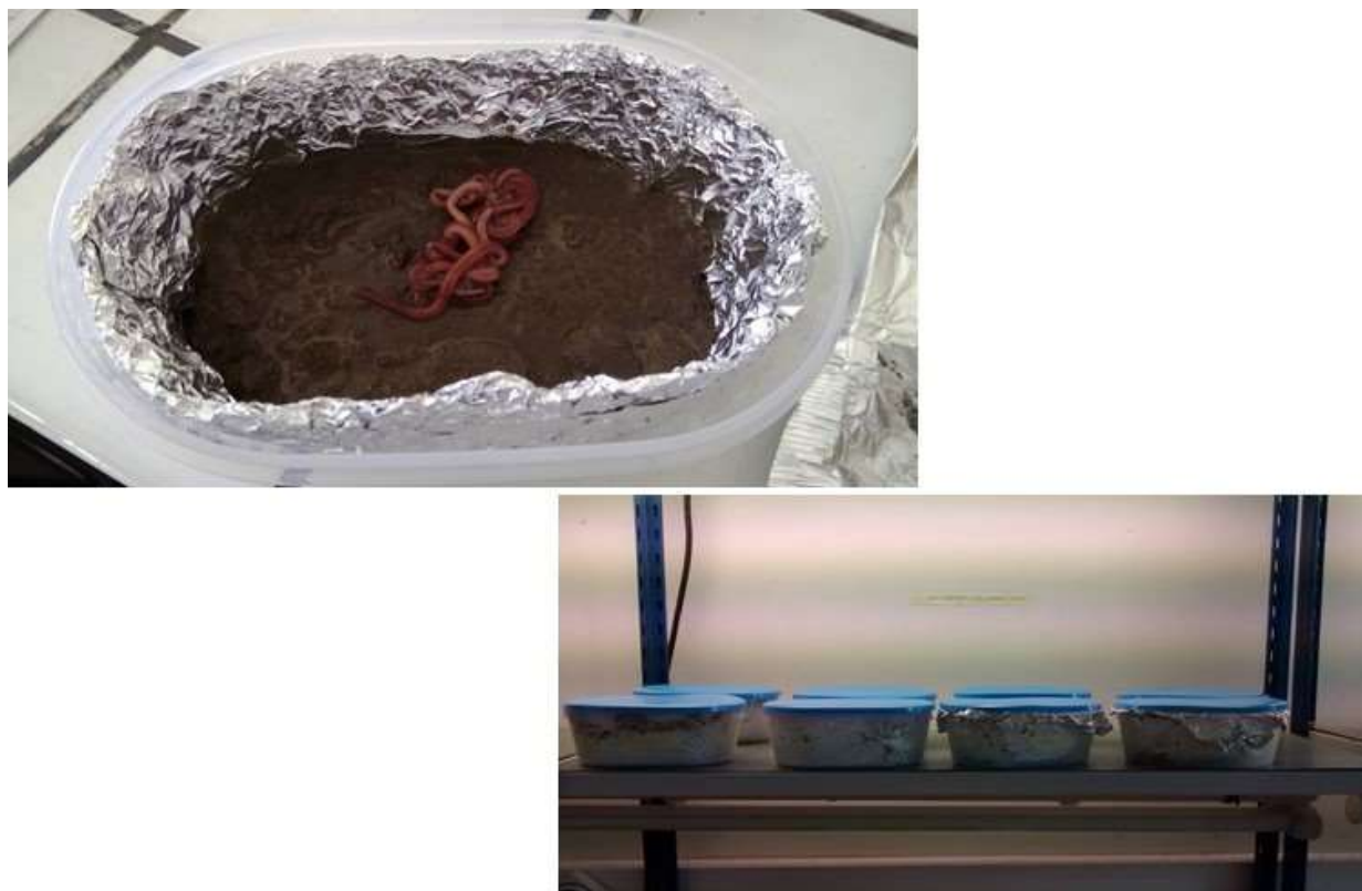
Figure 8 – Experimental system used for E. fetida reproduction and bioaccumulation tests.
