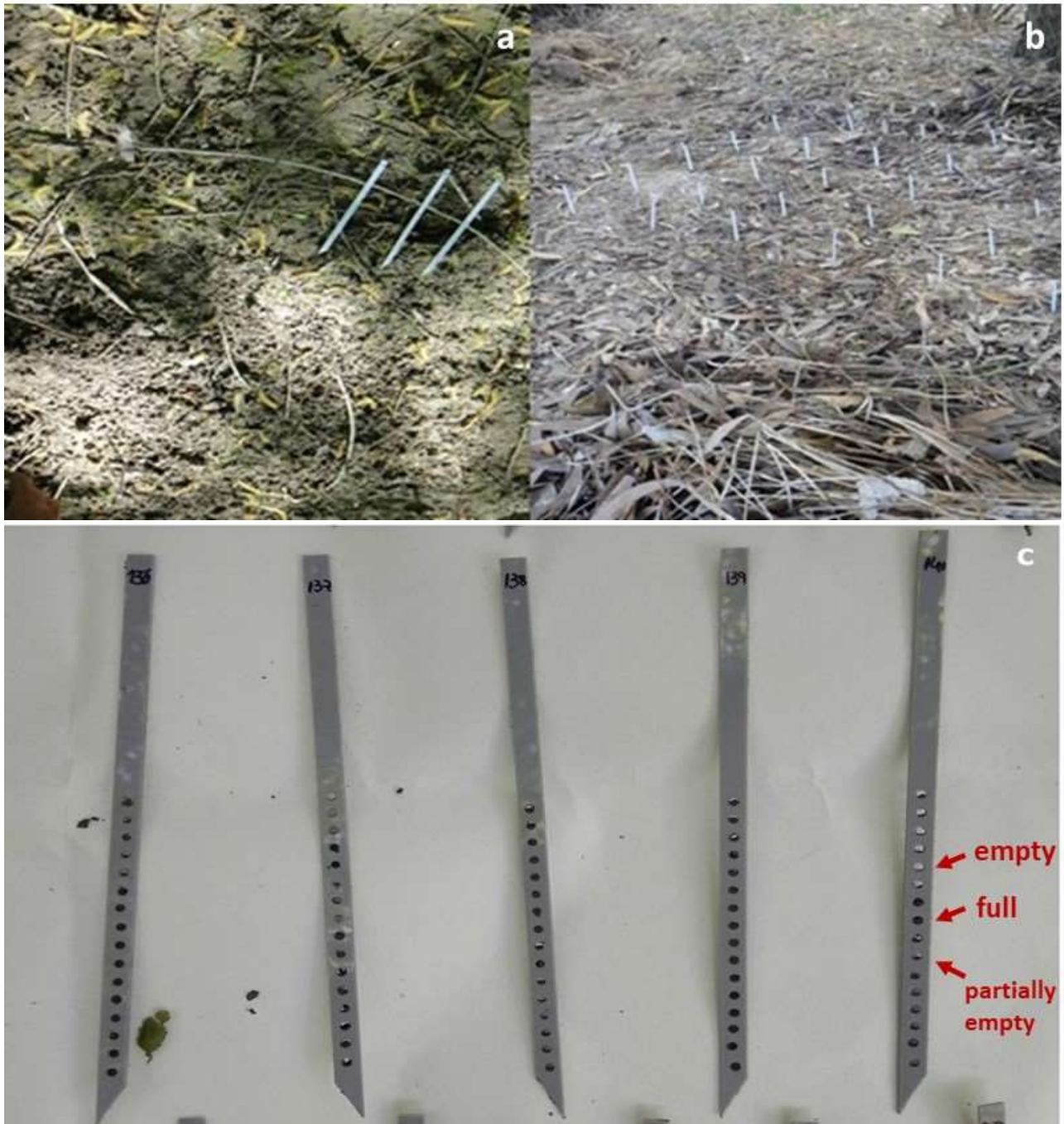
Figure 15 – Bait-lamina© test apparatus: (a) lamina-bait strips; (b) strips in the soil; (c) strips after collection from the soil.
