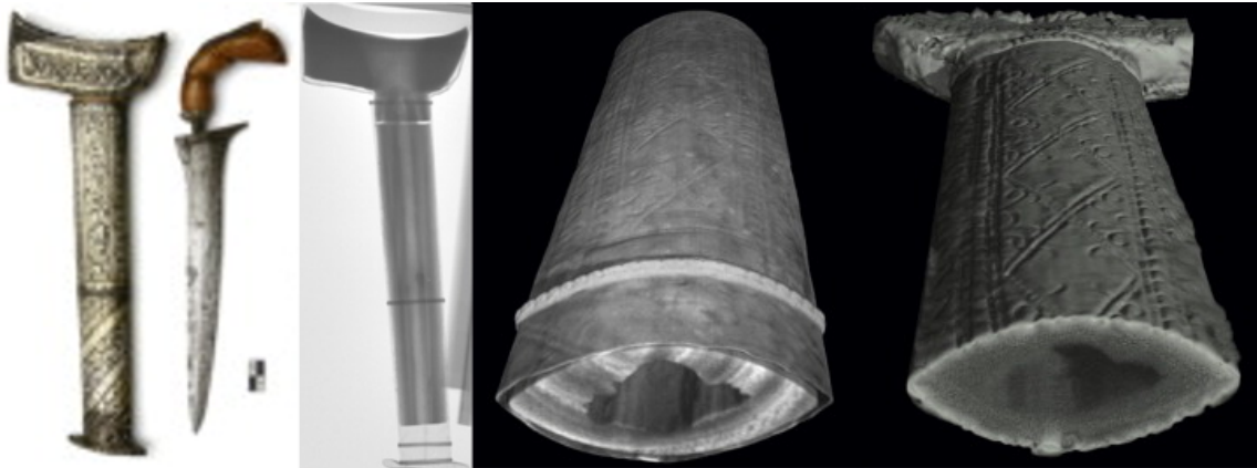
Figure 1.1 – Neutron and X-ray radiography of a dagger sheath. From left to right: the imaged sheath, neutron transmission image, neutron tomography and X-ray tomography [10]
