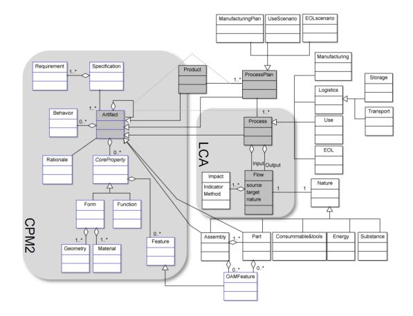
Figure 3.5 The CPMe<sup>3</sup> extension to support eco-design (Kozemjakin da Silva et al., 2013)
