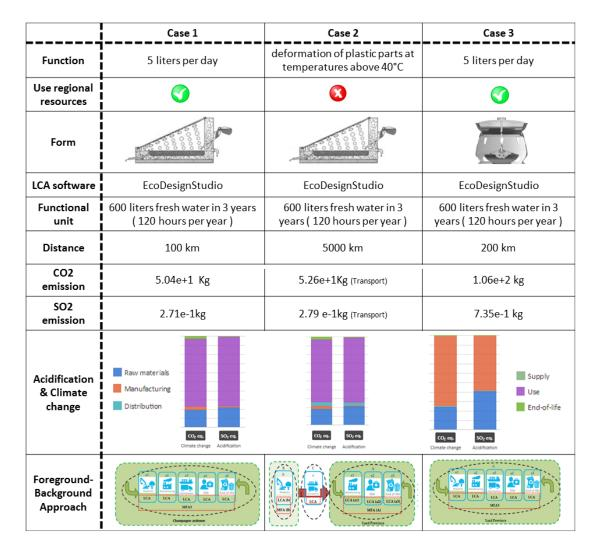
Figure.5.11. Comparisons between Eliodomestico and Solar Tears
