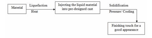
Figure 4.6 Simplified Manufacturing Process of a flashlight
