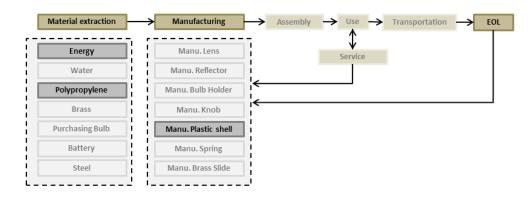
Figure 4.4 Life cycle stages for a simple flashlight
