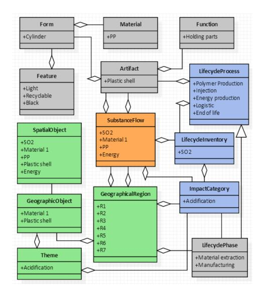
Figure 4.9 Class diagrams for plastic shell production
