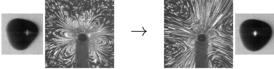
Figure 3.12: Example of one bubble whose pattern changes from a confined lobe pattern to a large pattern while the bubble is diminishing in size. Its radius diminishes from  $R_0 = 69.3\ \mu\text{m}$  to  $68.9\ \mu\text{m}$ , which despite the larger error margin supports the tendency of a shrinking bubble.
