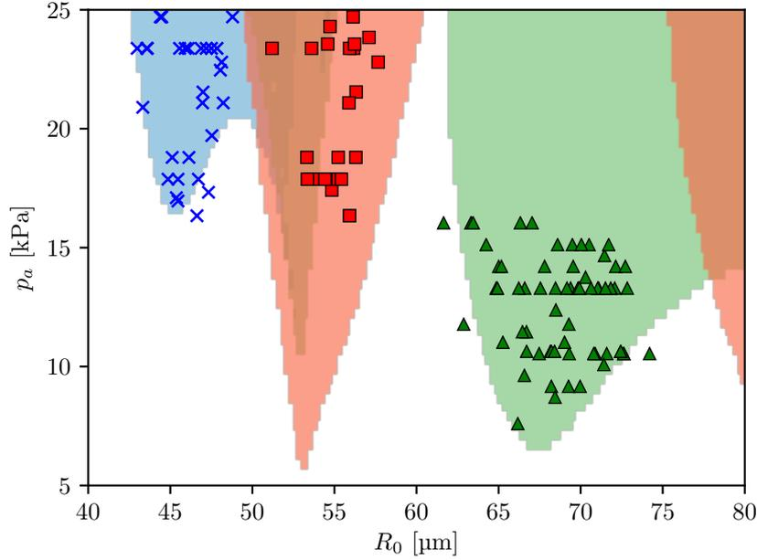
Figure 3.4: Pressure-radius map presenting experimental results classified according to the predominant mode of deformation ( $\times$  – mode 2,  $\triangle$  – mode 3,  $\square$  – mode 4. ) superimposed on numerically computed unstable areas (background colours: blue – mode 2, green – mode 3, red – mode 4).
