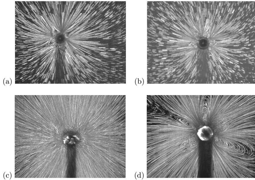
Figure 3.14: Streaming patterns for less well controlled bubbles. The frame size is  $1200\ \mu\text{m} \times 900\ \mu\text{m}$  for all subfigures; (a) approximately 0.2 s of streaming around a bubble oscillating on a mode 4, (b) approximately 0.1 s of streaming around a bubble probably oscillating on a mode 3, (c) approximately 1.2 s of streaming around a bubble oscillating on a mode 3 and (d) approximately 0.6 s of streaming around a bubble probably oscillating on a mode 3
