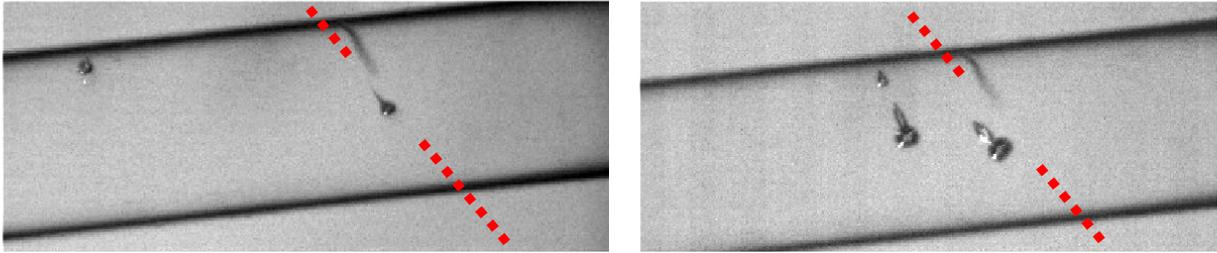
Figure A.4: Two examples of topview images; *left*: bubble is not influenced by other cavitation events and is jetting in the direction of the ultrasound propagation (red dotted line, the gap corresponds approximately to the frame of view of the side view camera); *right*: the jet is deviated due to the presence of other bubbles. Frame size for both is about  $1670\ \mu\text{m} \times 700\ \mu\text{m}$ .
