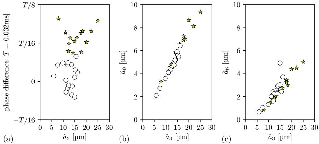
Figure 3.13: Study of amplitude and phasing for bubbles oscillating predominantly on a mode 3 and separated in large patterns –  $\star$  and lobe pattern –  $\circ$ . The  $x$ -axis of all three subplots is the maximum modal amplitude  $\hat{a}_3$ , the  $y$ -axis shows (a) the phase difference between  $a_0$  and  $a_6$ , (b) the maximum modal amplitude  $\hat{a}_0$  and (c) the maximum modal amplitude  $\hat{a}_6$ .
