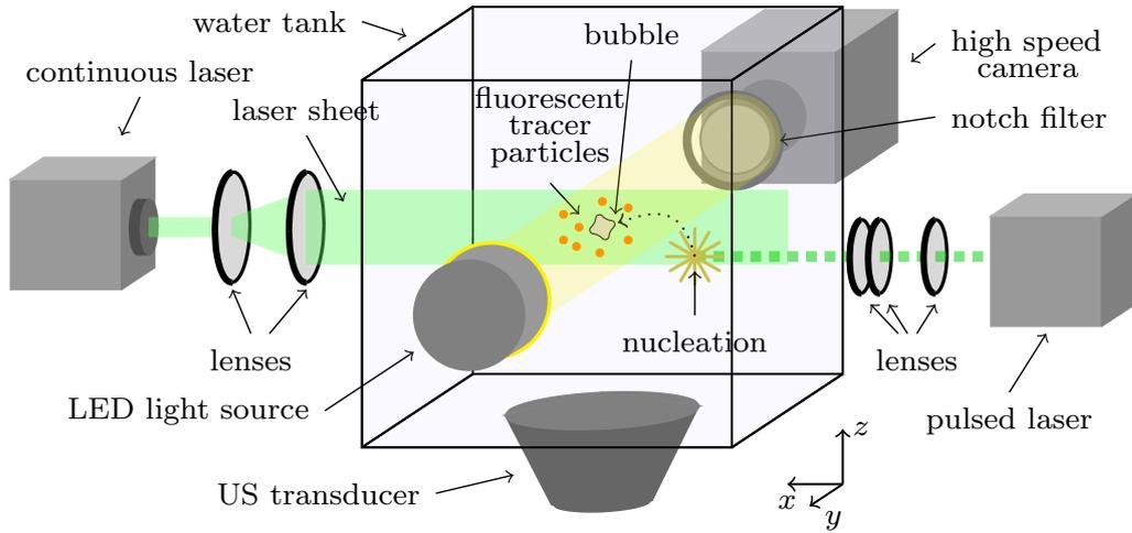
Figure 3.1: Experimental setup for the observation of microstreaming.
