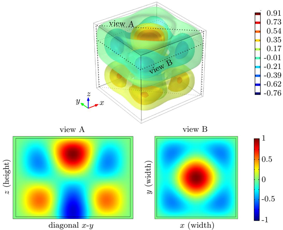
Figure 2.6: Simulation of the instantaneous acoustic pressure inside the cubic tank with inner dimensions of 8 cm. *Top*: iso-pressure in a 3D view, *bottom*: pressure distribution in the two planes through the pressure maximum (view B at a height of  $z \approx 6.4$  cm). Note that all pressures are normalized by the maximum pressure and that both high positive and high negative pressure values of the instantaneous field correspond to pressure maxima.
