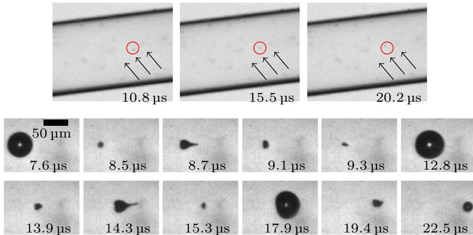
Figure A.8: Repeated on-axis jetting at 0.7 MPa peak negative pressure. The *upper row* shows the top view imaging, where a forward movement becomes visible. The arrows indicate the direction of the ultrasound wave. Note that the moments at which the top view was taken do not correspond to moments of maximum expansion. The two *lower rows* show chosen snapshots of the side view imaging, where repeated jetting becomes obvious.
