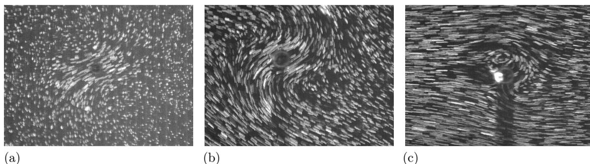
Figure 3.15: Fluid motion observed due to a bubble oscillating and at the time translating at a modulated frequency of (a) 781.25 Hz, (b) 15.625 Hz and (c) 156.125 Hz. The frame size is  $1200 \mu\text{m} \times 900 \mu\text{m}$  and the recording length 1.2 s for all subfigures.
