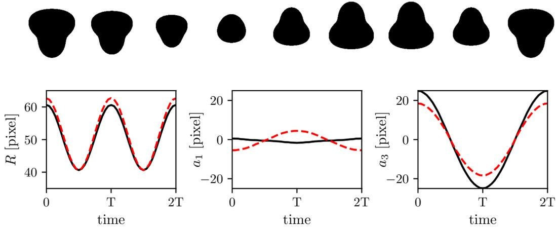
Figure 2.16: Simulation of a bubble oscillating on a mode 3 over two acoustic periods  $T$ , the axis of symmetry is turned  $20^\circ$  into the paper sheet. *Above*: snapshot series of the numerically created projection; *below*: red dashed line, temporal modal decomposition of the here presented bubble; black continuous line, temporal modal decomposition of a correctly oriented bubble.
