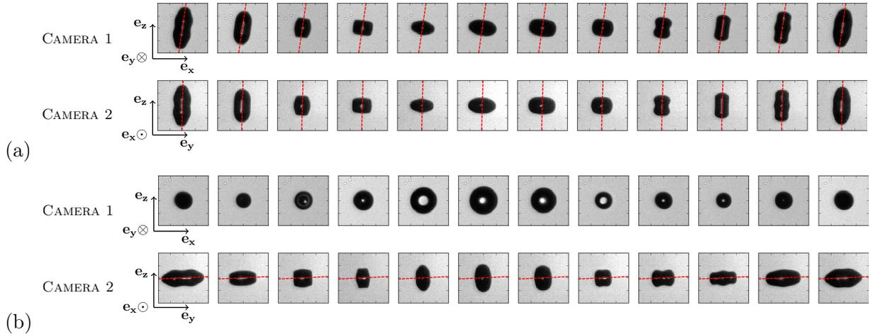
Figure 2.17: Two examples of bubbles recorded with two cameras; (a) the axis of symmetry equals the  $z$ -axis, the two cameras record the same information; (b) the axis of symmetry equals the  $y$ -axis, the camera 2 records the correct shape mode dynamics, while camera 1 records the oscillations of a seemingly spherical bubble.
