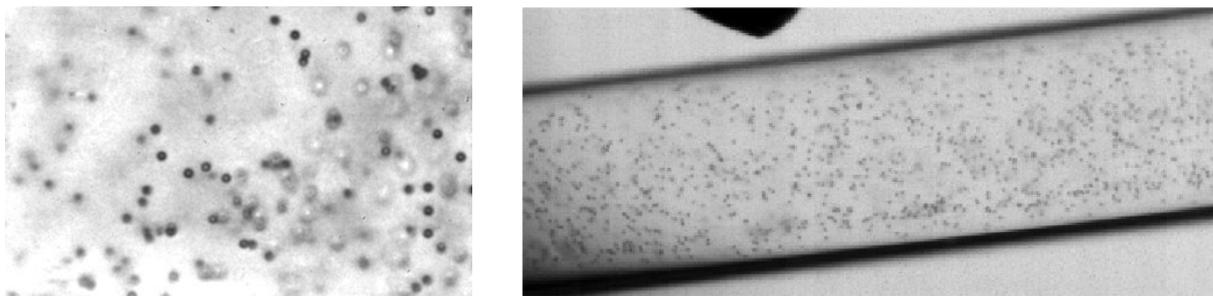
Figure A.3: Snapshots of  $7.5\ \mu\text{m}$  diameter beads, *left*: side view (camera 1, frame size  $435\ \mu\text{m} \times 270\ \mu\text{m}$ ) and *right*: top view (camera 2, frame size  $1670\ \mu\text{m} \times 700\ \mu\text{m}$ ). In the top view image, a part of the hydrophone tip can be seen.
