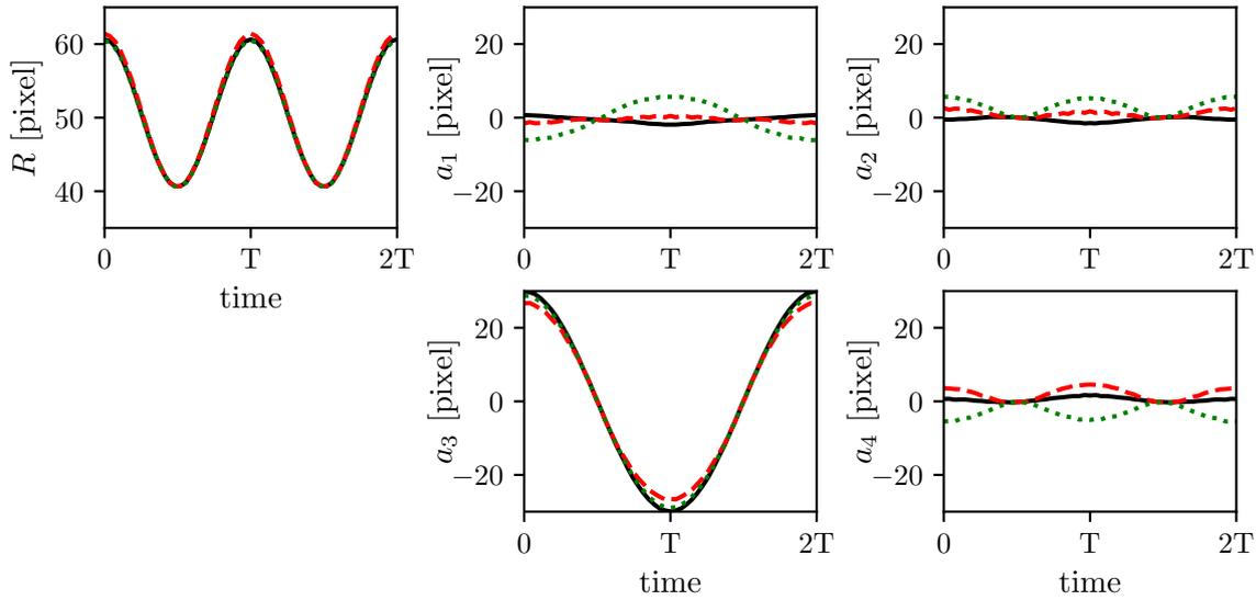
Figure 2.15: Modal decomposition of the bubble from figure 2.14 (b). The first four modal amplitudes are presented over two periods of oscillation  $T$  of the radial mode. Black continuous line, evaluation of the theoretical bubble shape; red dashed line, evaluation of the theoretical projection; green dotted line, evaluation of the projection when assuming the volume center as center of the projected shape.
