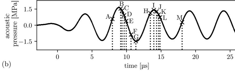
Figure A.2: Hydrophone signal at the focal spot for a transducer voltage set to 1.5 mV peak-peak. The letters indicated here are references for the snapshot series shown in figure A.5.
