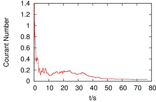
FIGURE 6.1: Temporal evolution of Courant number for  $\alpha = 0.3$ . After a certain early moment, the Courant number is smaller than 0.5, thereby confirming that the temporal resolution is sufficient.
