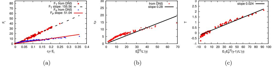
FIGURE 5.6: Determination of the model parameters (a)  $\beta_P, \beta_T$  (b)  $d'_P$  and (c)  $\zeta'$  by linear regression of the DNS data.
