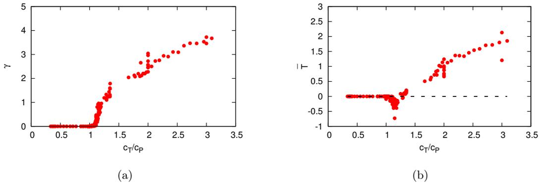
FIGURE 5.2: (a) Ratio between the energy components time-averaged during the steady state,  $\gamma = \bar{E}_T/\bar{E}_P$ , plotted as a function of the forcing parameters ratio,  $c_T/c_P$ , for the complete set of simulations. (b) Transfer from the toroidal to the poloidal energy components,  $\bar{T} = \langle u_\theta^2 u_r/r \rangle$ , plotted as a function of  $c_T/c_P$ .
