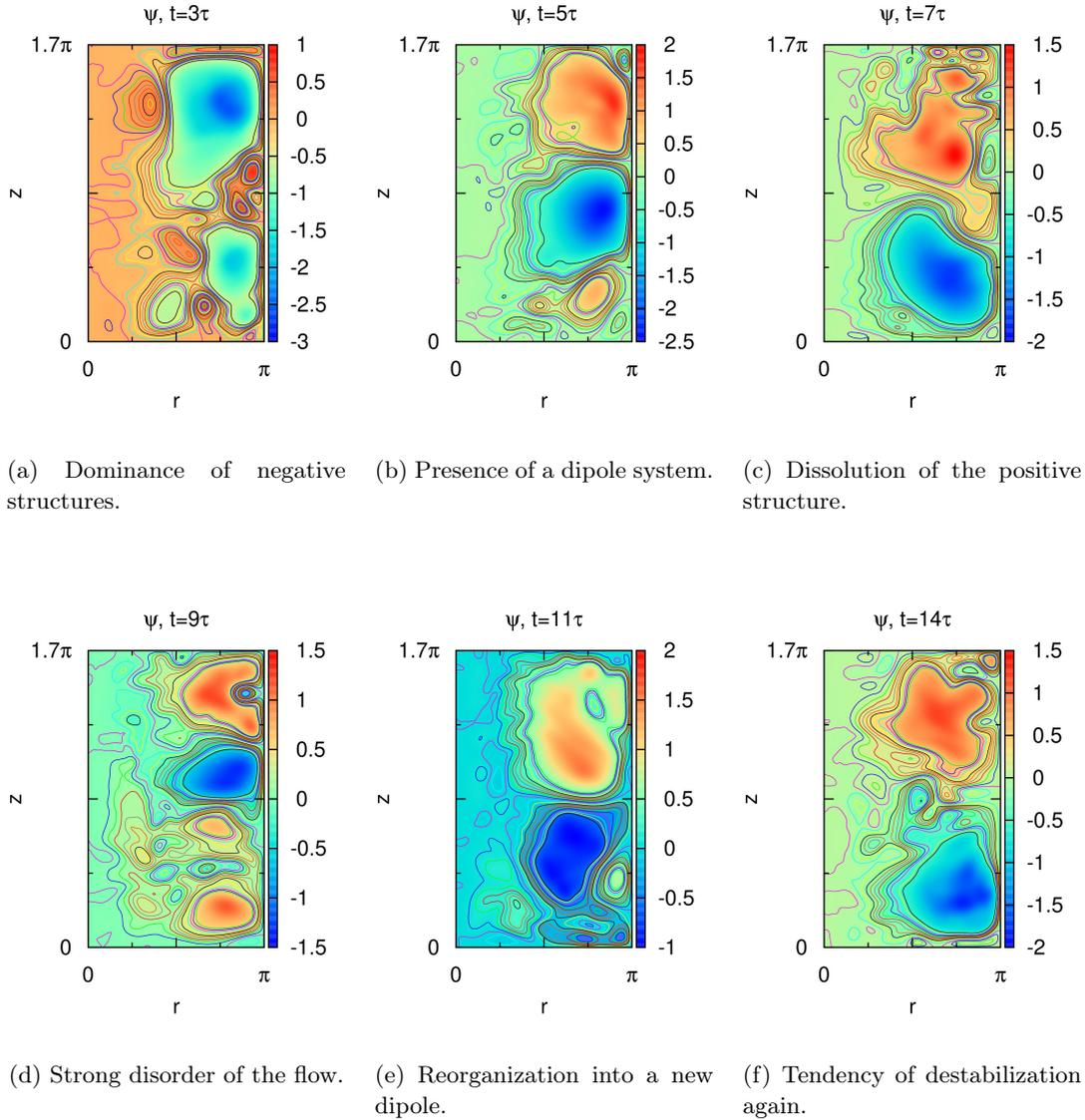
FIGURE 4.2: Contour plots of the stream function  $\psi$  within the poloidal plane  $(r, z) \in [0, R] \times [0, H]$  at different times. Both emergence and dissolution of big structures can be observed.
