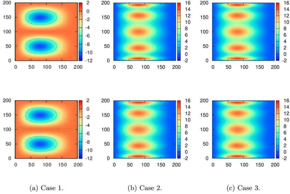
FIGURE 3.2: Comparison of the stream function  $\psi$  in the three cases detailed in Tab.3.1. With naked eye, original (top) and recomposed (bottom) fields show no difference for Cases 1 and 3, while they are slightly different close to the top and bottom of the cylinder for Case 2 due to insufficiency of vertical resolution.
