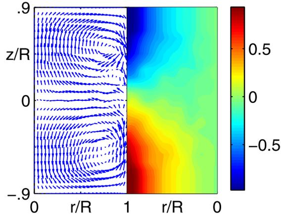
FIGURE 4.12: Pictures cited from [21] showing time-averaged fields. Time-averaged  $\psi$  and  $u_\theta$  for  $\text{Re}_\Omega = 2.5 \times 10^5$ . The arrow plot represents the  $\bar{\psi}$  field and the colored contour displays the  $\bar{u}_\theta$  field.
