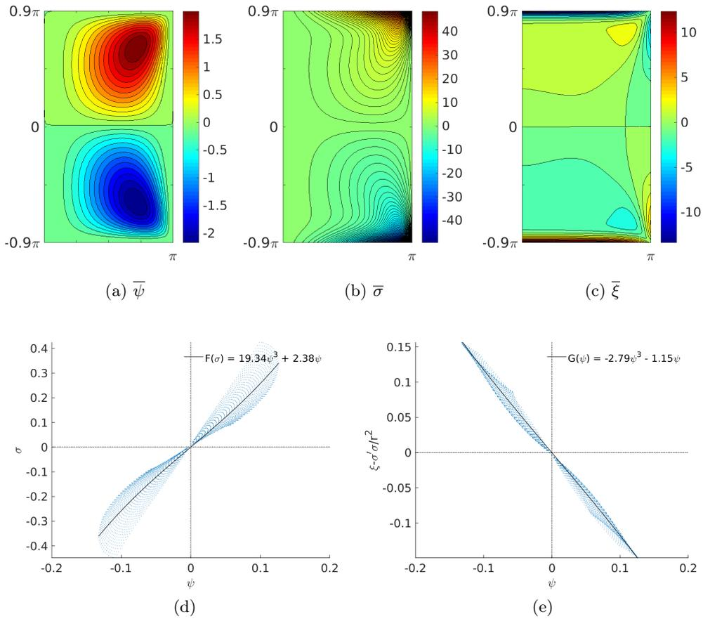
FIGURE 4.14: Time-averaged  $\psi$ ,  $\sigma$  and relationships  $\bar{\sigma} = F(\bar{\psi})$  and  $\bar{\xi} - \bar{\sigma}'\bar{\sigma}/r^2 = G(\bar{\psi})$  during the stationary state for  $\text{Re}_\Omega = 250$ . The scatter plots of functions  $F$  and  $G$  consider only the points within the bulk of  $(r, z) \in [0, 0.81R] \times [-0.56H/2, 0.56H/2]$ .
