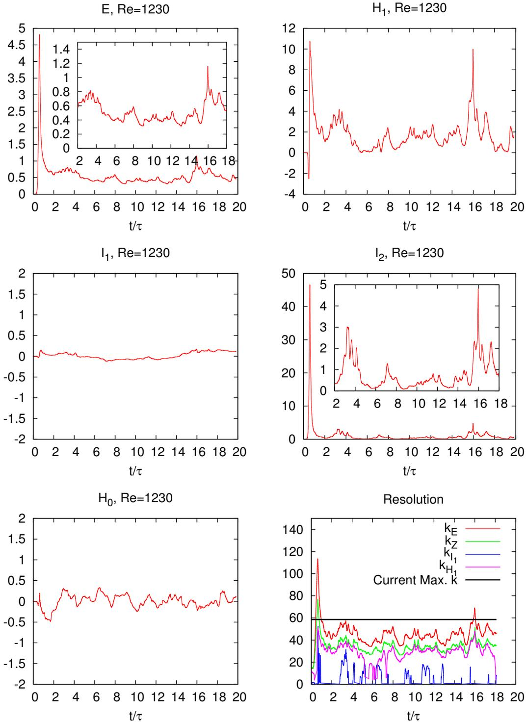
FIGURE 4.1: Temporal signals of statistical invariants and resolution tests for a forced simulation. In this simulation, velocity fields of  $2\tau \leq t \leq 15\tau$  are considered stationary and are thus used.
