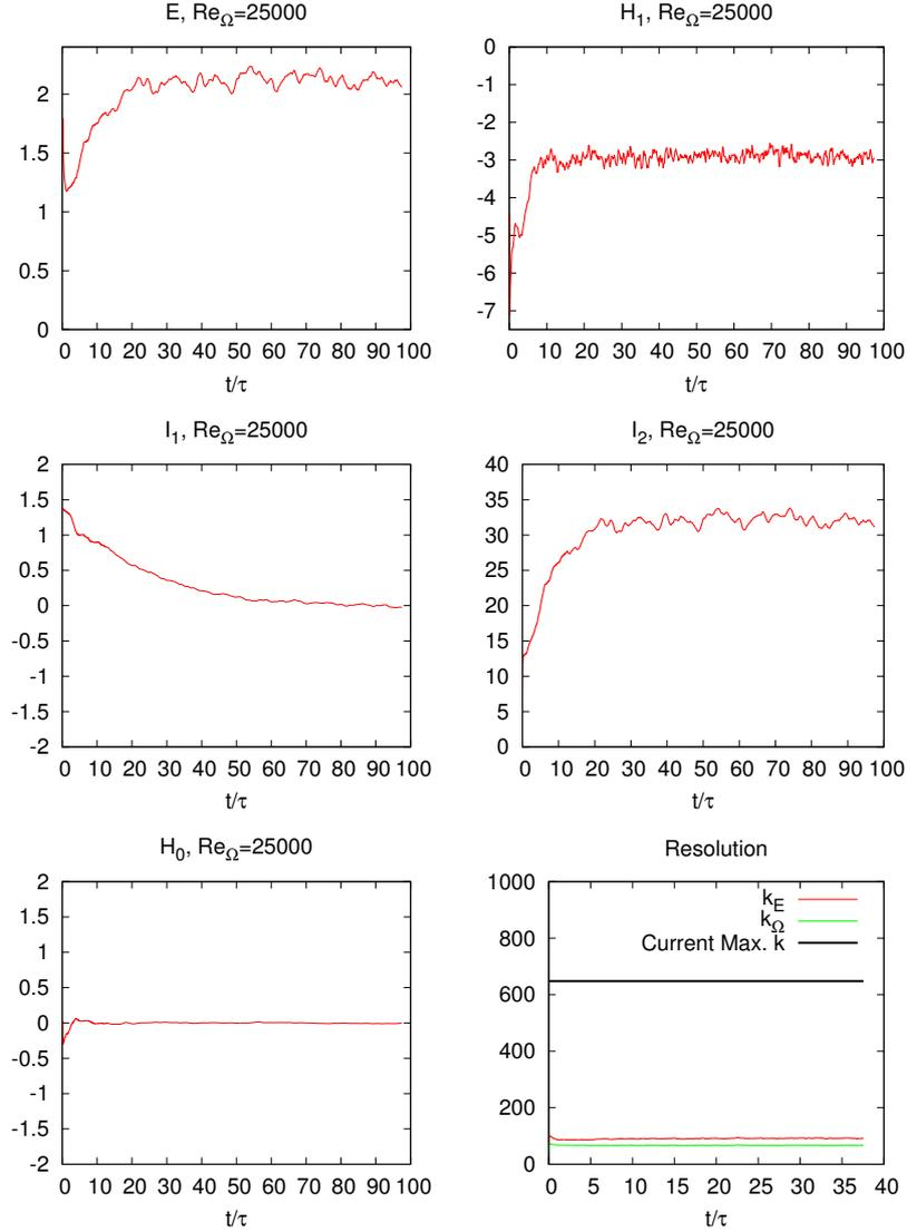
FIGURE 4.8: Temporal signals of statistical invariants and resolution tests for a forced simulation. As explained in Appendix C, the dissipation rate of  $I_1$  and  $H_1$  in a mechanically forced case are not well defined, and hence only the energy and enstrophy dissipation rates are used to check the resolution.
