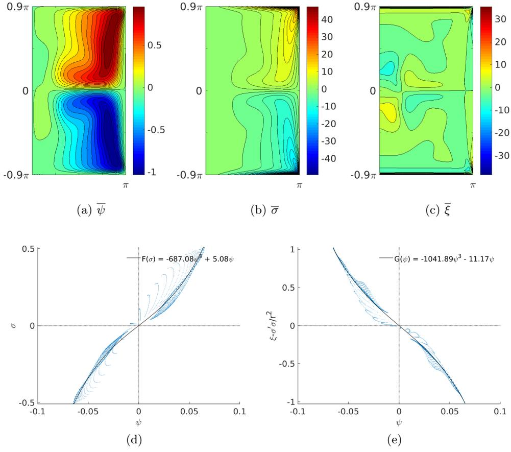
FIGURE 4.13: Time-averaged  $\psi$ ,  $\sigma$  and relationships  $\bar{\sigma} = F(\bar{\psi})$  and  $\bar{\xi} - \bar{\sigma}'\bar{\sigma}/r^2 = G(\bar{\psi})$  during the stationary state for  $\text{Re}_\Omega = 2500$ . The scatter plots of functions  $F$  and  $G$  consider only the points within the bulk of  $(r, z) \in [0, 0.81R] \times [-0.56H/2, 0.56H/2]$ .
