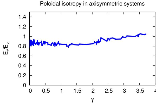
FIGURE E.1: Ratio of  $E_r/E_z$ . The energy isotropization between the radial and axial directions can be observed : as  $\gamma$  increased, the ratio is stabilized around 1 though it has a slight rising tendency for large  $\gamma$ .
