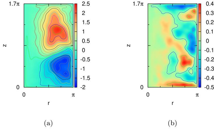
FIGURE 5.3: Contour plots of the time-averaged poloidal stream function  $\psi$  defined as :  $u_r = -\partial_z \psi / r$ ,  $u_z = \partial_r \psi / r$ . The average is performed during the statistically steady state. The time interval over which  $\psi$  is averaged is (a)  $4 < t/\tau < 16$  and (b)  $9 < t/\tau < 22$ . Forcing parameters are : (a)  $c_P = 3$ ,  $c_T = 1$  ( $c_T/c_P = 1/3$ ) and (b)  $c_P = 1.2$ ,  $c_T = 3.6$  ( $c_T/c_P = 3$ ).
