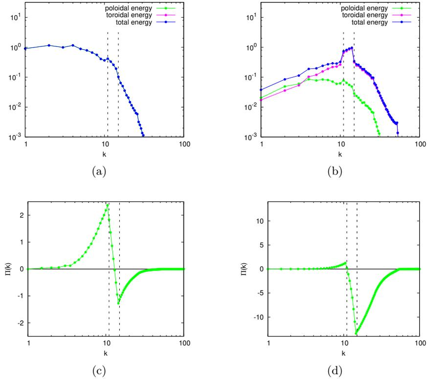
FIGURE 5.4: Time-averaged (a,b) energy spectra of the total, poloidal and toroidal energy, and (c,d) energy flux. Values of the forcing parameters : (a,c)  $c_P = 3$ ,  $c_T = 1$  ( $c_T/c_P = 1/3$ ), (b,d)  $c_P = 1.2$ ,  $c_T = 3.6$  ( $c_T/c_P = 3$ ). The vertical dashed lines indicate the range of wave-numbers in which forcing is applied.
