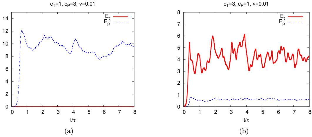
FIGURE 5.1: Time evolution of the poloidal and toroidal energy components for : (a)  $c_P = 3$ ,  $c_T = 1$  ( $c_T/c_P = 1/3$ ) and (b)  $c_P = 1$ ,  $c_T = 3$  ( $c_T/c_P = 3$ ). Time is normalized by  $\tau = R/(2\bar{E}/3)^{1/2}$ , where  $\bar{E}$  is the total kinetic energy of the flow time-averaged in the statistically steady state.
