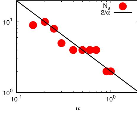
FIGURE 6.3: Number of lobes observed in the kinetic energy visualization in the horizontal median plane of the cylinder, for different values of  $\alpha$ . The trend is reproduced by the function  $N_s = 2/\alpha$ .
