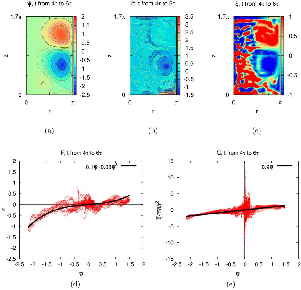
FIGURE 4.4: Time-averaged  $\psi$ ,  $\sigma$  and relationships of  $\bar{\sigma} = F(\bar{\psi})$  and  $\bar{\xi} - \bar{\sigma}'\bar{\sigma}/r^2 = G(\bar{\psi})$  during  $4\tau \leq t \leq 6\tau$ . The scatter plots of functions  $F$  and  $G$  consider only the points within the bulk of  $(r, z) \in [3R/16, 7R/8] \times [H/16, 15H/16]$ .
