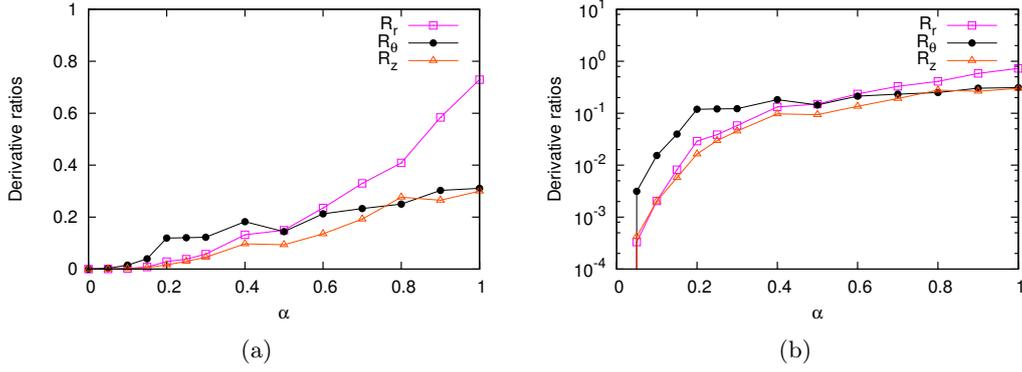
FIGURE 6.5: Axisymmetry level described by the ratios  $\mathcal{R}_r$ ,  $\mathcal{R}_\theta$ ,  $\mathcal{R}_z$ . For  $\alpha = 0$ , the three ratios are 0, as expected due to the axisymmetry constraint. (a) linear-linear scale; (b) linear-log scale.
