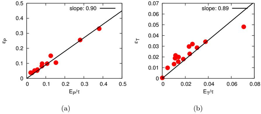
FIGURE 6.6: Scatter plots of dissipation rates to extract dissipation coefficients  $d_P$  and  $d_T$ . The linear fittings show that the model (6.20,6.23) for the dissipation rates appears to work well.
