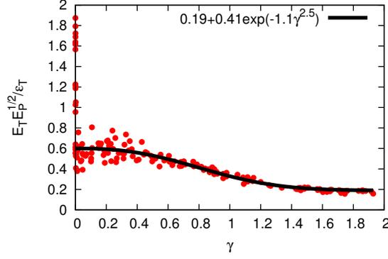
FIGURE 5.5:  $E_T E_P^{1/2} / \epsilon_T$  calculated by DNS, plotted as a function of  $\gamma$  (red dots). The (black) line shows the best data fitting  $0.19 + 0.41 \exp(-1.1\gamma^{2.5})$ . Following Eq.(5.13), this fitting provides an estimate of  $L' = L/d_T$ .
