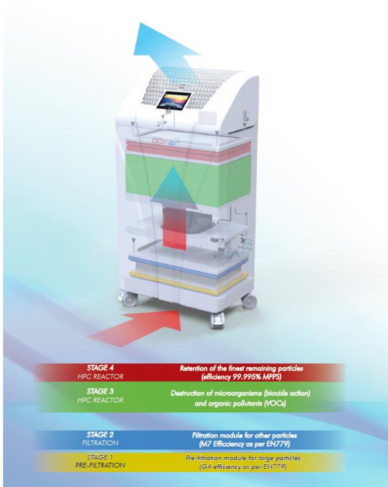
Figure 84 : Representation of Room DOPair showing the air flow and the various air cleaning stages [27]
